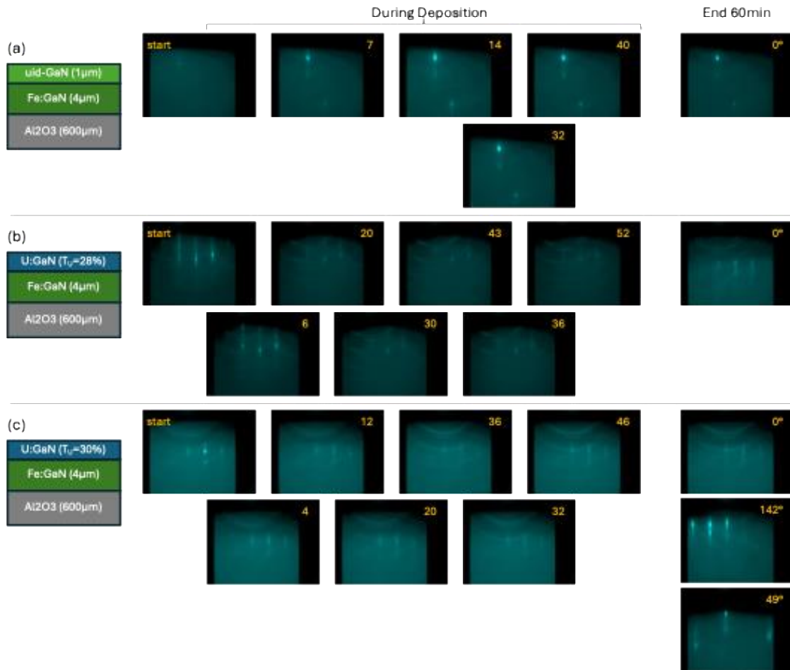
Figure S5.3 – Schematics and RHEED images for (a) uid-GaN, (b) OP%=28, and (c) OP%=30. The yellow number in the top corner of each image denotes the time elapsed throughout the growth for each image. The rightmost images show RHEED patterns taken at the end of growth, labeled with optional rotations relative to the starting image shown.
