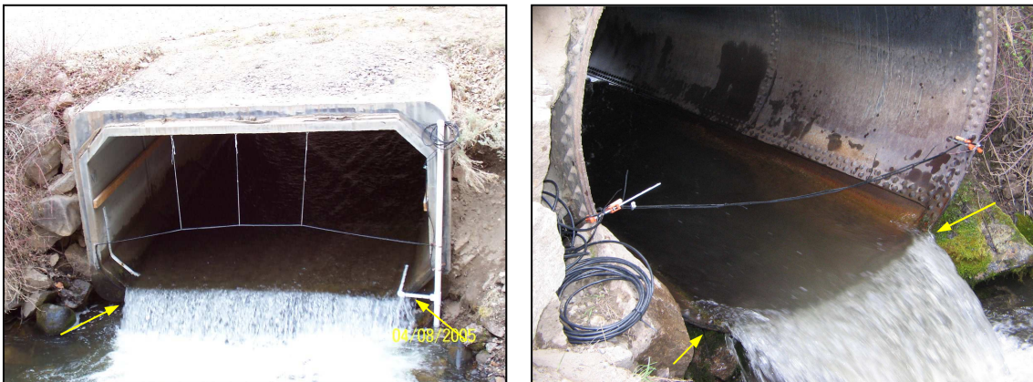
Figure 5. Antenna construction design for culverts where the antenna could be mounted directly on the downstream outlet of the culvert. Left: outlet of culvert 1. Right: outlet of culvert 4. Arrows indicate location of lower end of antenna loop.
