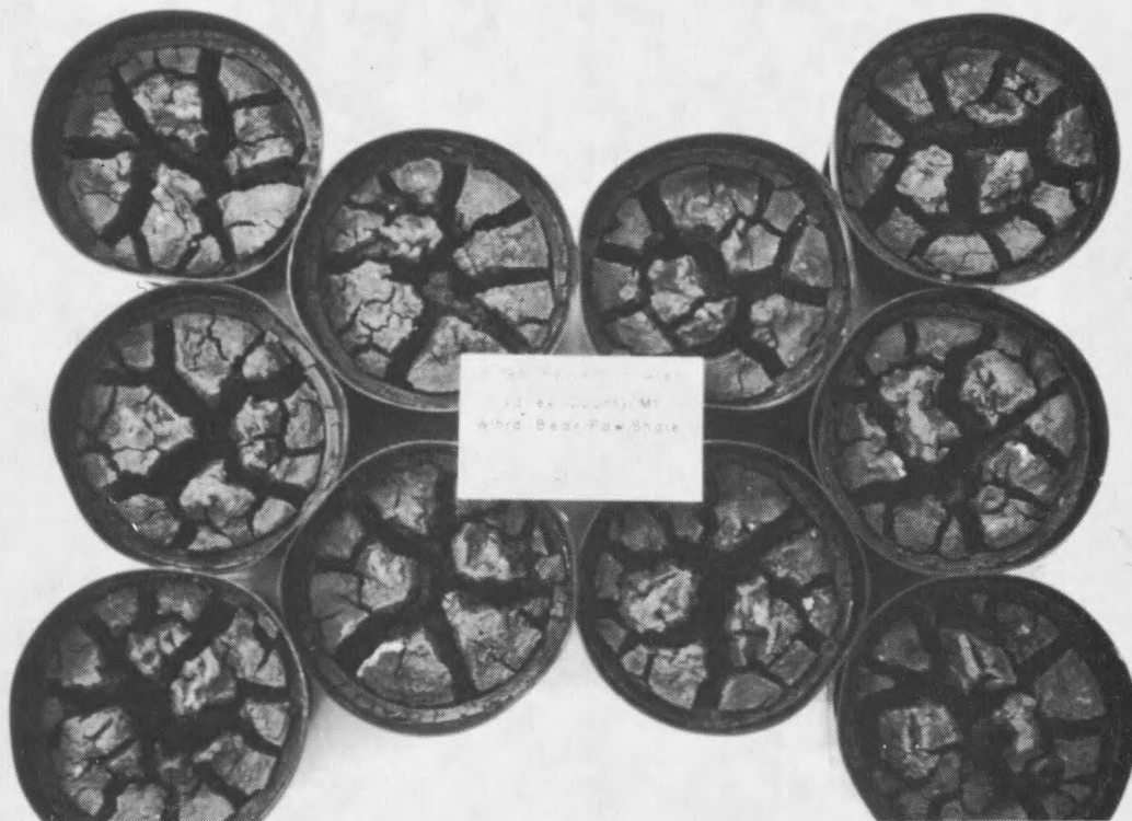
Figure 2. Cracks which formed in a soil weathered from Bear Paw Shale.
