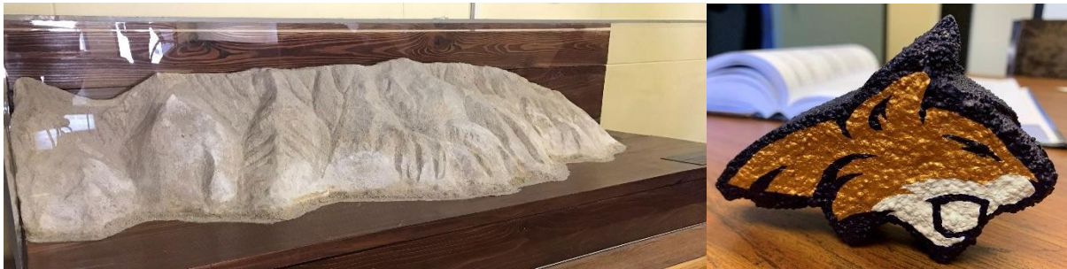
Figure 2.12: (Left) 0.9 m x 0.3 m x 0.3 m Biomineralized replica of the Bridger Mountain Range. (Right) Biomineralized replica of the Montana State University mascot, the Bobcat.
