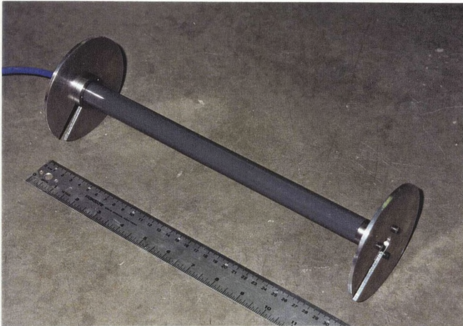
Figure 10. Vibrating Wire Embedment Displacement Gauge
