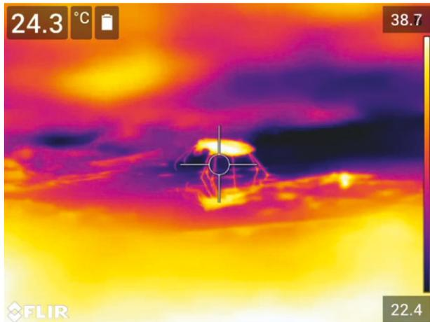
**Fig. 1.** A still image from the thermal video recording. The reflection of the beetle on the substrate is the more accurate surface temperature of the substrate not influenced by solar reflection and was the target area for measurement when analyzing the temperature-time relationship data in the recordings. Video still by JL Bowley.
