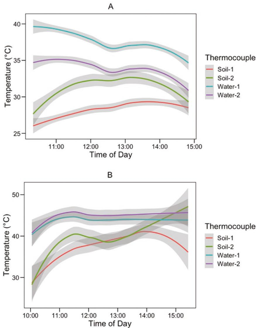
**Fig. 6.** A) Average temperatures during periods of observation at Dragon Spring recorded by thermocouples. B) Average temperatures during periods of observation at Rabbit Creek recorded by thermocouples.
