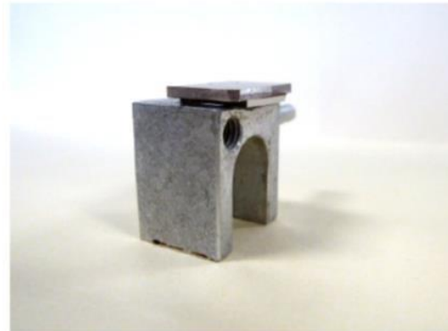
Figure 30. Epoxy Sandwich Mounting Method for Sample Preparation (Gill, 2014)
