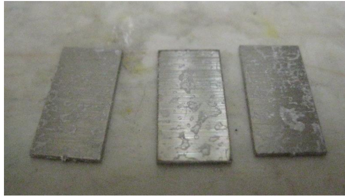
Figure 23. Ni-201 Samples Coated with 1 \text{ mgcm}^{-2} \text{ Na}_2\text{SO}_4
