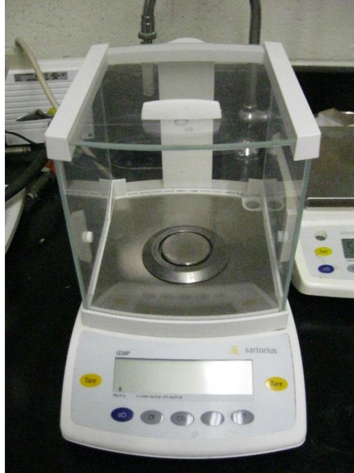
Figure 22. Sartorius Model LE26P Balance for Mass Measurements
