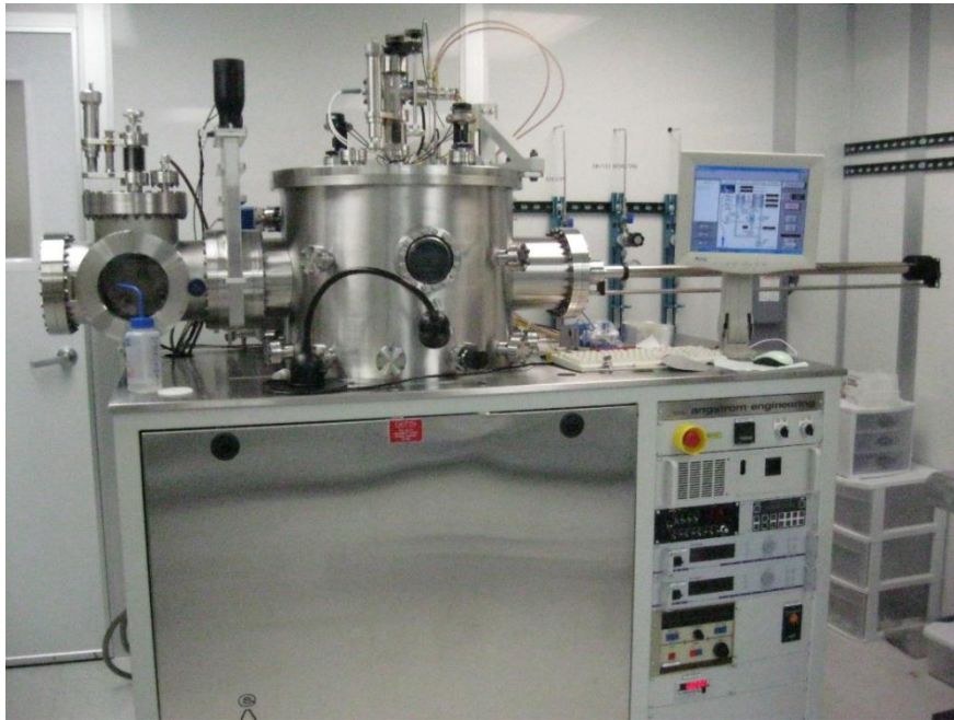
Figure 20. Angstrom Magnetron Sputtering System for Thin Film PVD
