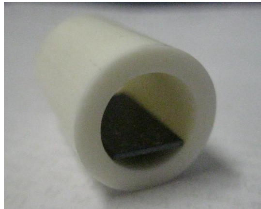
Figure 24. Samples in Alumina Tube Crucibles for Exposure Testing
