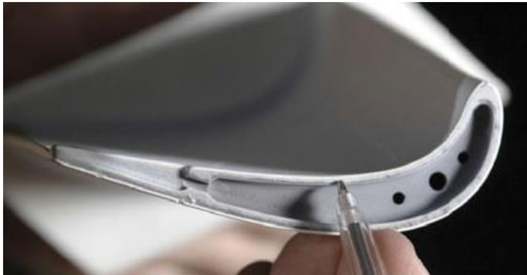
Figure 10. 300 \mu m Stamm Coating for Gas Turbine Blades (Saini, 2012)
