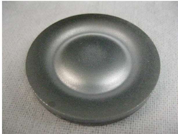
Figure 19. Racetrack Region of a Chromium Target in Magnetron Sputtering
