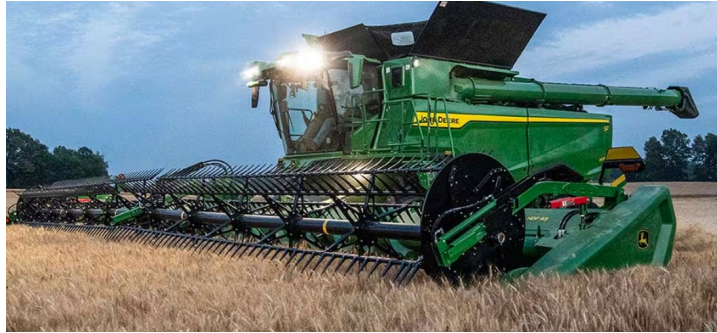
Figure 1-3: Conventional draper header used for cereal grain harvest ( https://www.deere.com/en/harvesting/draper-platforms/ ).
