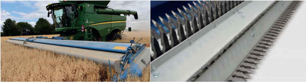
Figure 1-1: Stripper harvester attachment (left) and stripping rotor (right) ( https://www.shelbourne.com/harvest/stripper-header/ )
