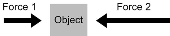
Which total force is equal to the two forces acting on the object?
