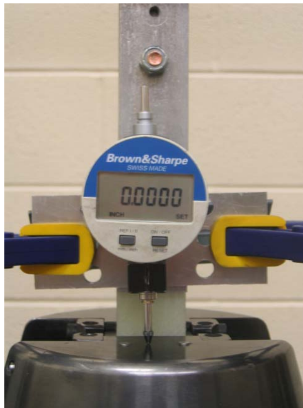
Figure 40. Bearing tension (BT) coupon test setup loaded in the grips of a uni-axial Instron test machine.
