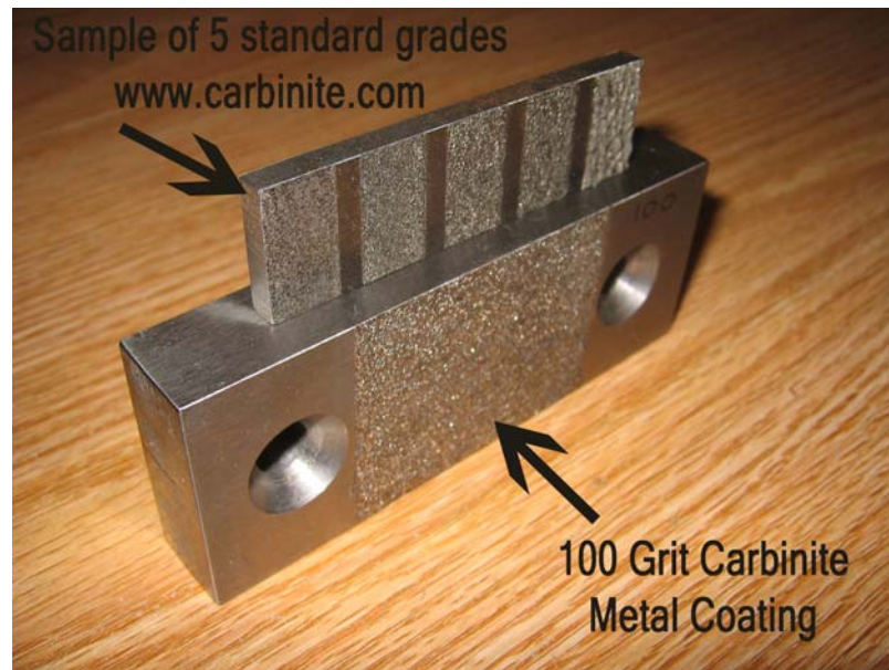
Figure 6. Carbinite coating provides an abrasive gripping surface for composite IPL test coupons.
