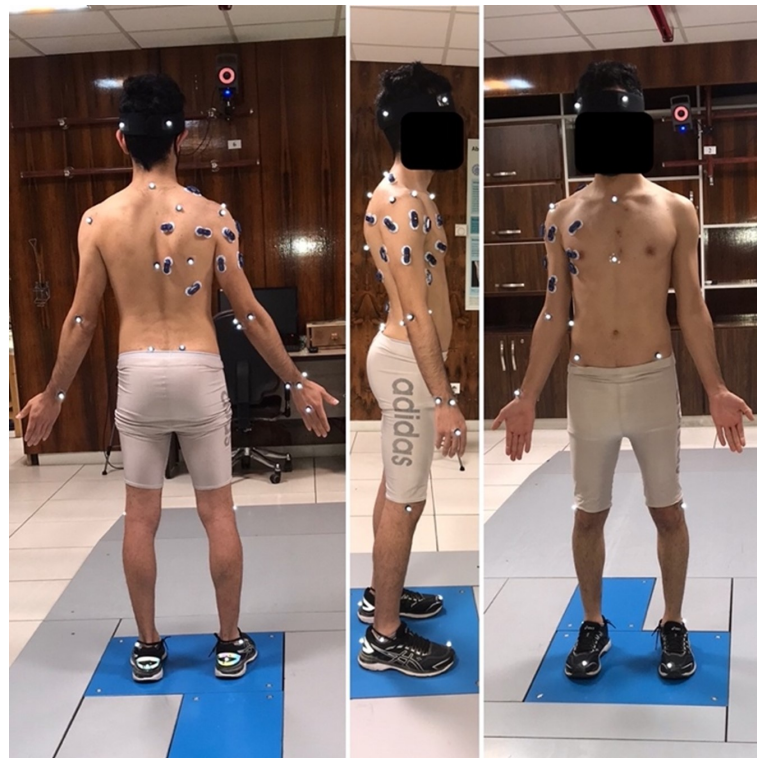
Figure 1. The surface reflective marker and EMG electrode placement for 14 muscles: anterior deltoid, middle deltoid, posterior deltoid, infraspinatus, upper pectoralis major, middle pectoralis major, lower pectoralis major, latissimus dorsi, triceps lateral, triceps medial, biceps brachii, upper trapezius, middle trapezius, and lower trapezius muscles in the motion analysis lab with ten high-speed motion Vicon cameras (Vicon Industries Ltd., Hampshire, UK).
