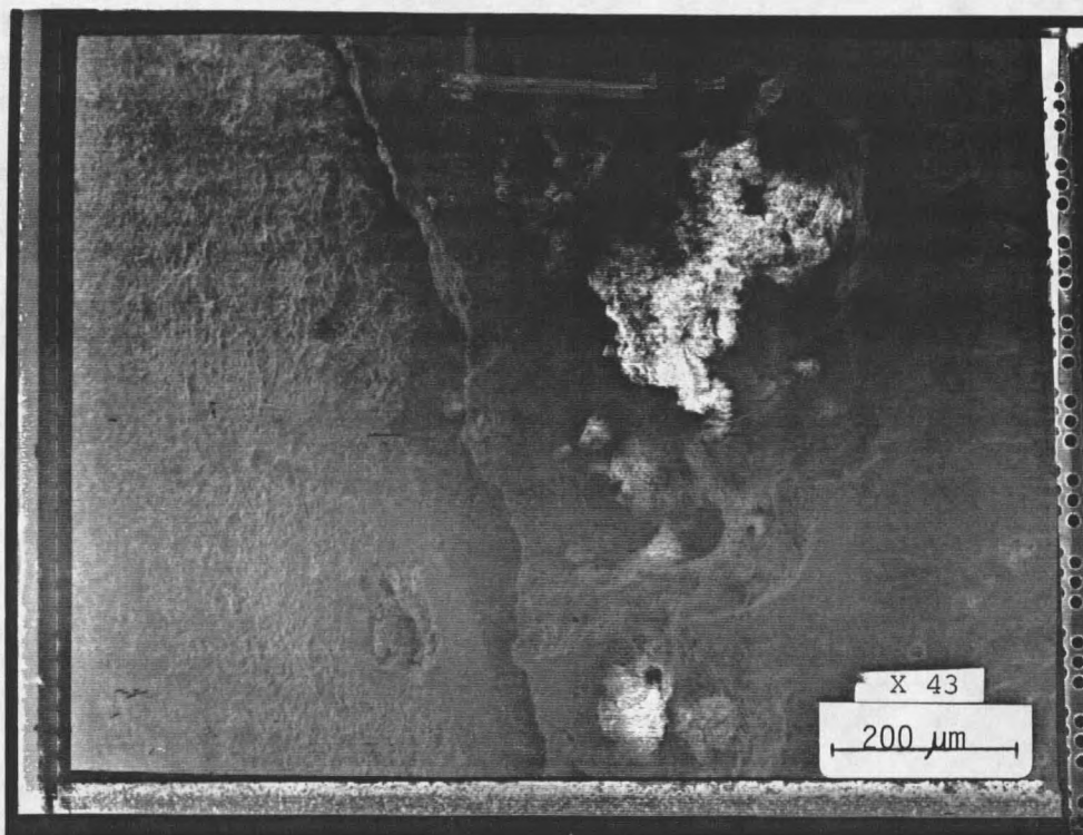
Figure 1. Scanning Electron Micrograph (SEM) of a corrosion pit from a section of 304 stainless steel heat exchanger tubing (x43) from a plant which has suffered similar problems (photograph provided by Tatnall, Dupont, Delaware).
