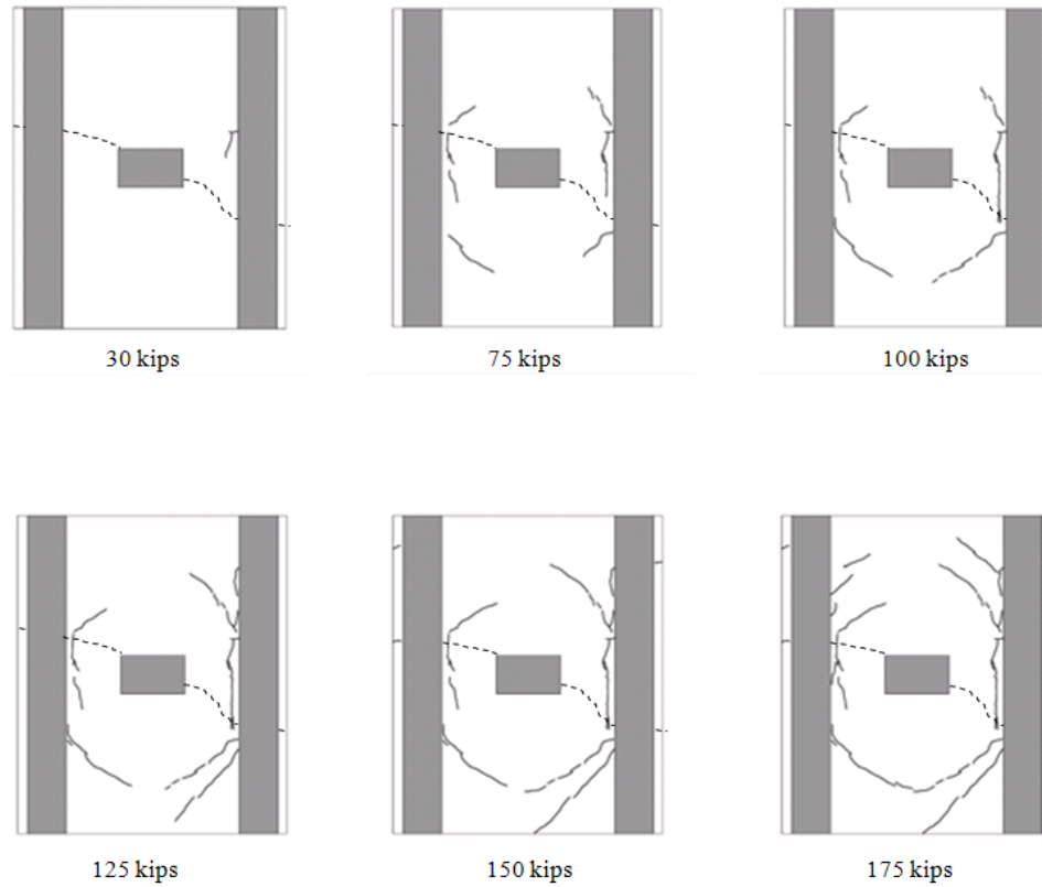
Figure 34: Evolution of Crack Patterns on Top Surface of Test Slab
