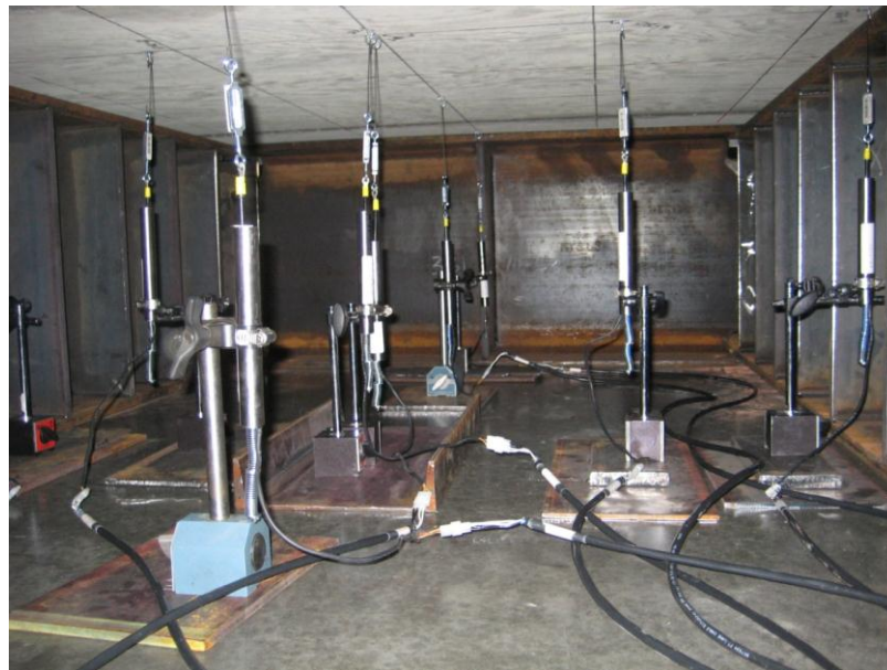
Figure 27: Photograph of LVDTs Under Test Slab
