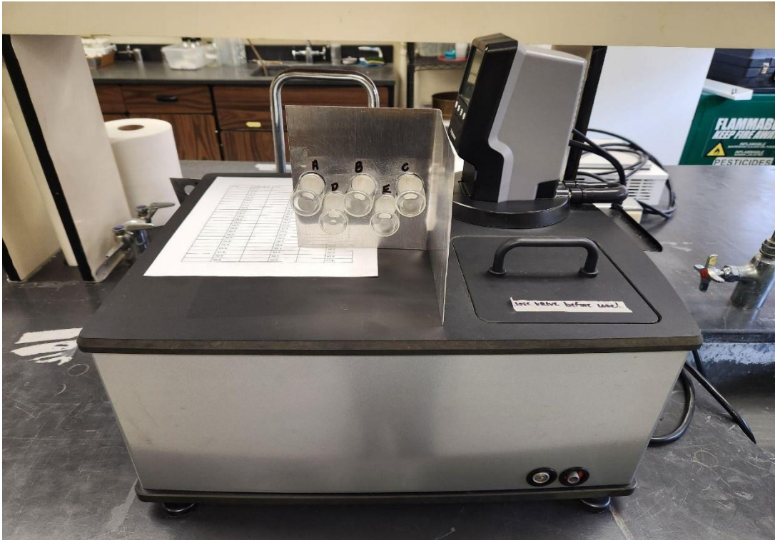
Figure 2. Critical thermal minimum ( CTL_{\min} ) ramping assay. Individual moth vials attached to aluminum sheet shown on top of programmable water bath.
