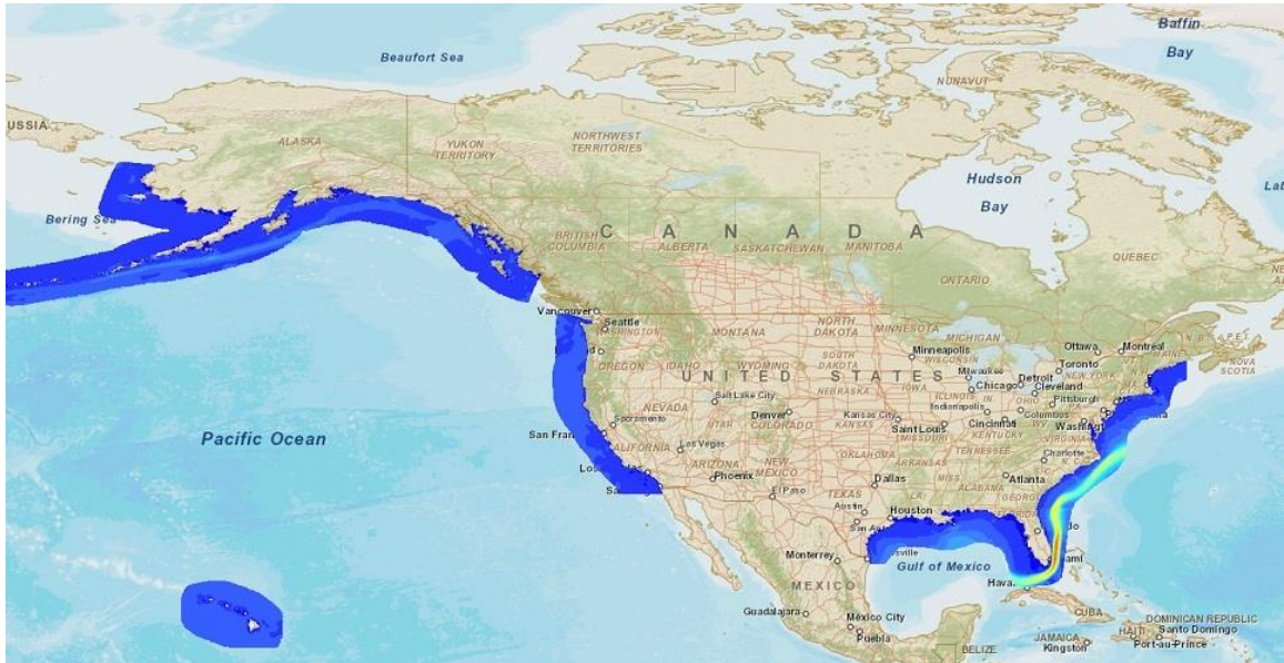
Figure 1. Areas near US coasts that possess high velocity ocean currents where energy extraction devices could be installed 1 .
