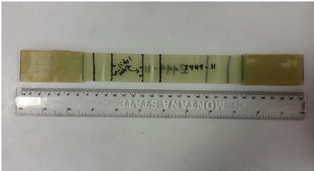
Figure 25. Coupon 2444-11 and the damage after the coupon was removed from the saltwater bath.
