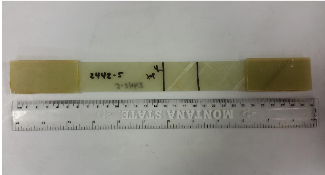
Figure 24. Coupon 2442-5 and the damage seen after the coupon was removed from the saltwater bath.
