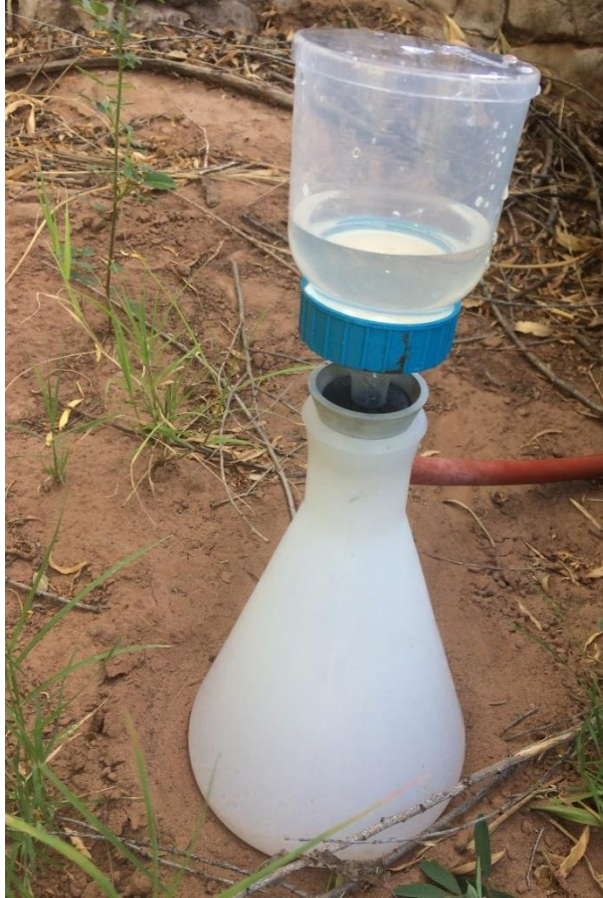
Figure 7. Sterile Nalgene analytical test filter funnel (RX Biosciences, Gaithersburg, MD).
