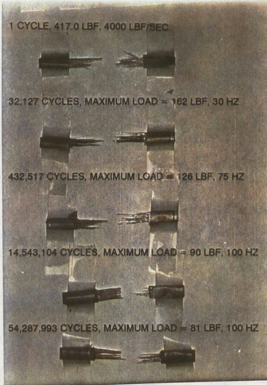
Figure 13. Photograph of typical broken specimens from different load levels and frequencies.
