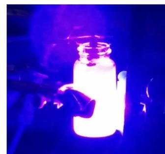
**Figure 6.** Phosphorescence of PtTFPP-painted vial. Shows emission in the red region.
