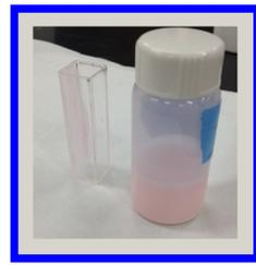
**Figure 3.** Cuvette with one surface covered in a layer of PtTFPP paint (left). Vial of PtTFPP paint (right) used to coat the surface of the cuvette.
