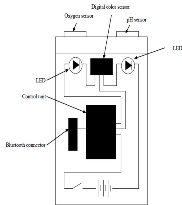
**Figure 1.** Schematic of optical pH/oxygen sensor.
