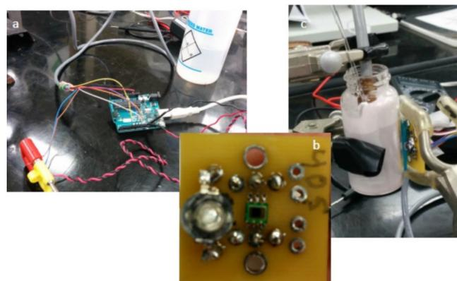
**Figure 4.** Set-up of oxygen-sensing component. Arduino board (a) attached to Hamamatsu Digital Color Sensor (b). LED emits 405 nm wavelength light onto PtTFPP-painted vial (c).
