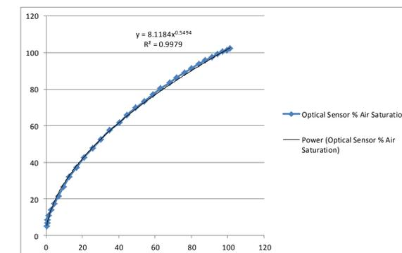
**Figure 9.** Power law fit curve between the percent air saturation values given by the Clark sensor and the optical oxygen sensor.
