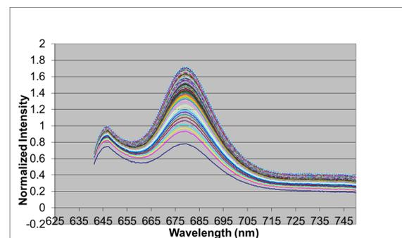
**Figure 5.** Emission Spectra of PtTFPP-containing paint over twenty minutes from air saturated (low amplitude,  $t = 0$  s), to zero oxygen (high amplitude,  $t=1200$  s).
