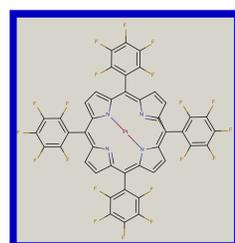
**Figure 2.** Platinum (II) meso-tetrakis (2,3,4,5,6 – penta-fluorophenyl) porphyrin (PtTFPP)
