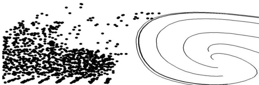
Figure 2. Streamlines were seeded in the flow on the downstream side of the biofilm from Figure 1b, and they show a recirculation-like pattern in the fluid flow.
