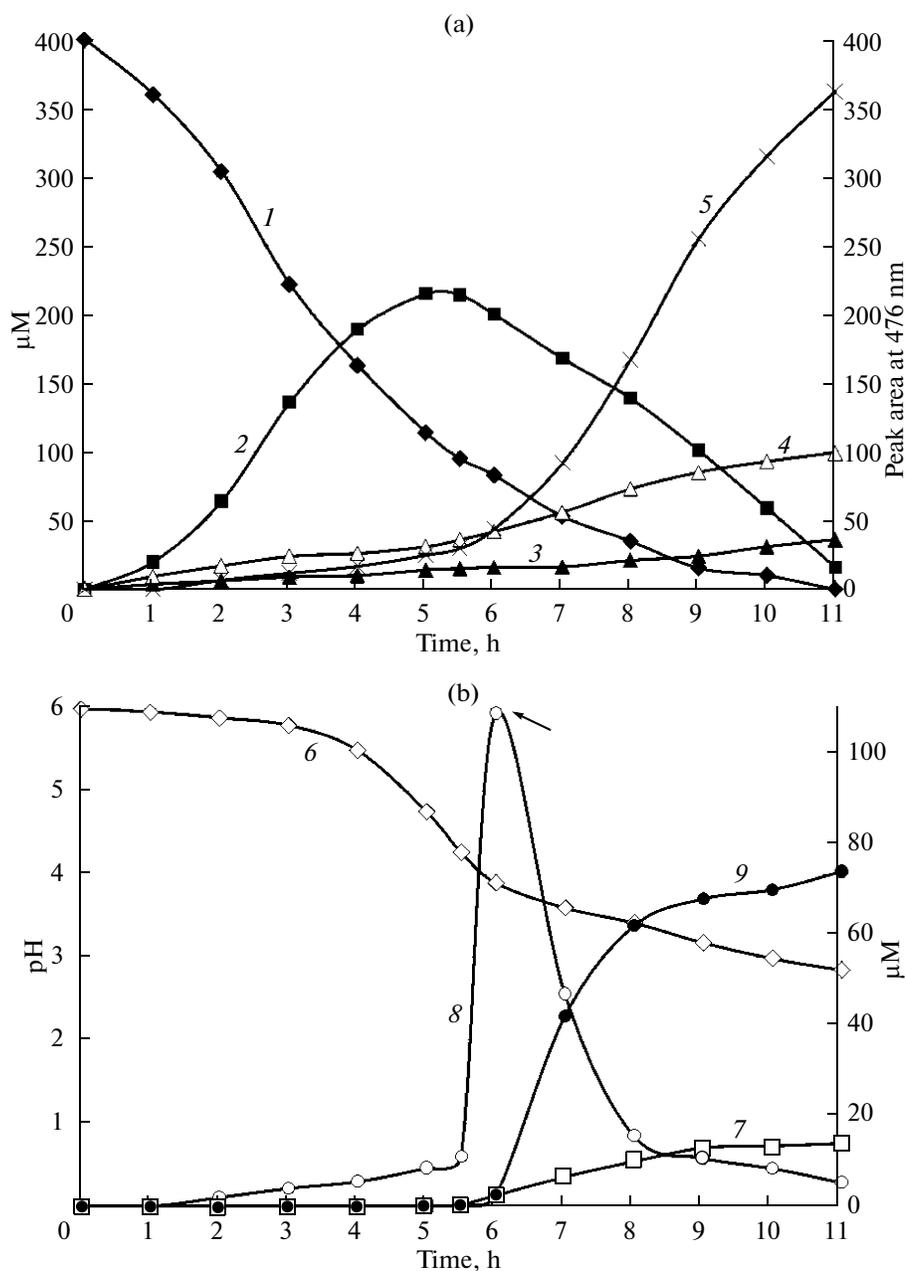
**Fig. 2.** Production of metabolites in the course of TNT transformation by *G. candidum* AN-Z4 under aerobic conditions at pH 6.0. At the stage of 2,4-DNT formation,  $\text{NaNO}_2$  (100  $\mu\text{M}$ ) was added into the medium as an additional source of nitrite ions (shown by the arrow). Curve designations as in Fig. 1.
