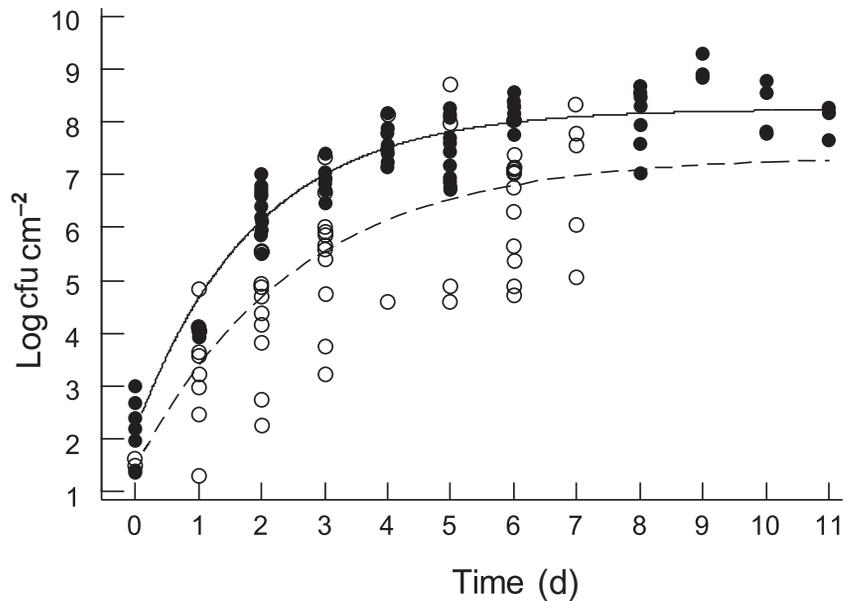
**Fig. 3** Comparison of biofilm accumulation curve for all untreated control reactors (●) and for all untreated toilets (○). The time scale is in days for the reactors and weeks for the toilets
