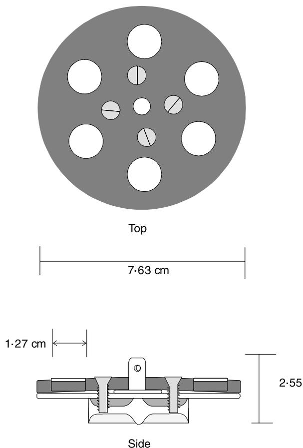
**Fig. 1** Rotating disc reactor rotor
