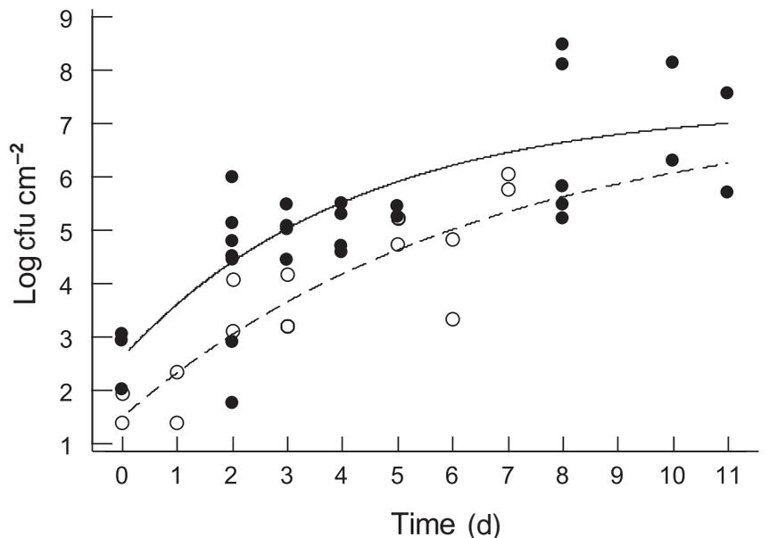
**Fig. 4** Comparison of biofilm accumulation curve for  $9 \text{ mg l}^{-1}$  chlorine-treated reactors (●) and for  $9 \text{ mg l}^{-1}$  chlorine-treated toilet (○). The time scale is in days for the reactors and weeks for the toilet
