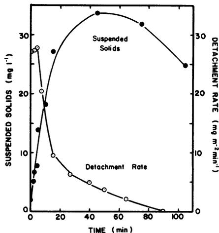
FIG. 2. Response of a biofouled tubular reactor to 1 mM EGTA (pH 7.5) addition at zero time (surface area of the reactor, 0.797 m<sup>2</sup>; volume, 10.49 liters; residence time, 2 h).
