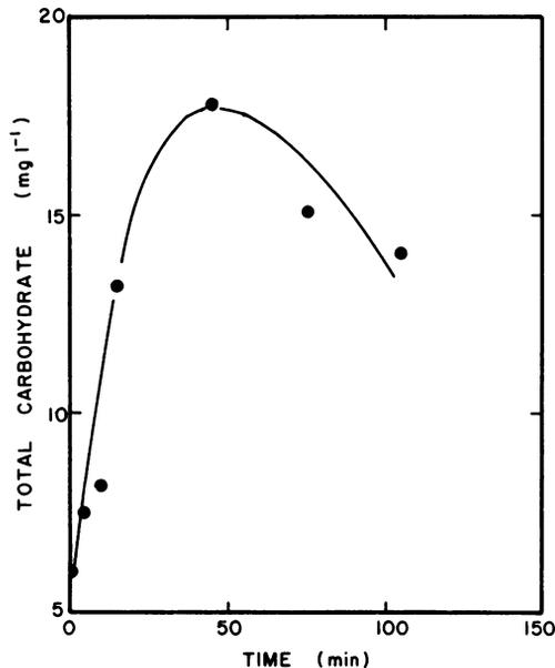
FIG. 4. Suspended total carbohydrate (as glucose equivalence) in effluent after addition of EGTA. Soluble effluent glucose concentration was less than 1 mg liter<sup>-1</sup>.
