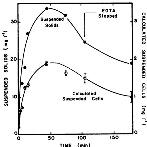
FIG. 3. Change in suspended solids and suspended cell mass in the effluent due to the addition of EGTA at zero time (error bars based on standard deviation from epifluorescent cell counts).
