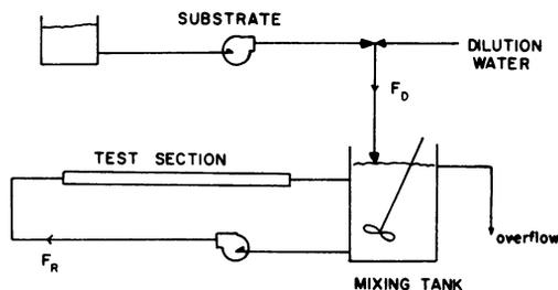
FIG. 1. A simplified flow diagram of a recycle tubular reactor (tube alloy A1-6X; influent glucose, 44.26 mg liter<sup>-1</sup>; NH<sub>4</sub>Cl, 0.159 mg liter<sup>-1</sup>; MgSO<sub>4</sub> · 7H<sub>2</sub>O, 0.44 mg liter<sup>-1</sup>; K<sub>2</sub>HPO<sub>4</sub>, 0.796 mg liter<sup>-1</sup>; KH<sub>2</sub>PO<sub>4</sub>, 0.133 mg liter<sup>-1</sup>).
