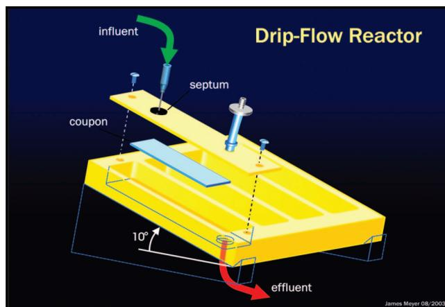
Figure 1. DFR used in biofilm-removal experiments.
