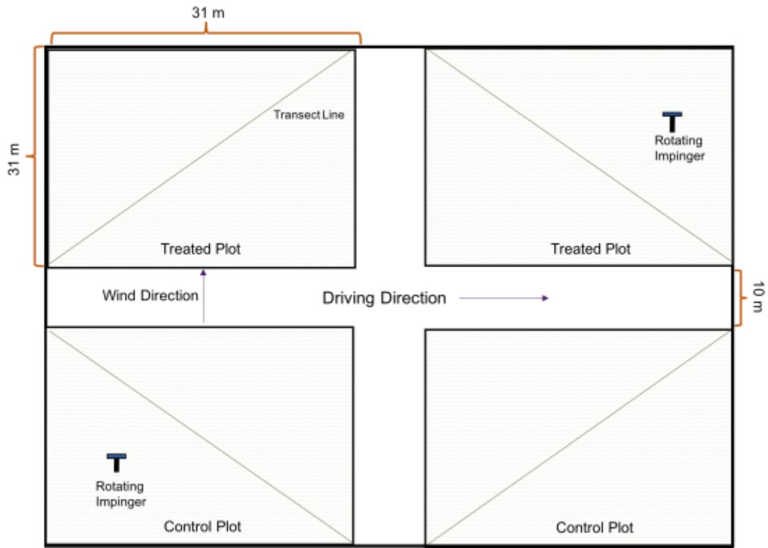
Figure 6. Diagram of an experimental plot used to collect alfalfa foliage. Each quadrat is 31 m x 31 m and intersected by a 10-m drive line. Rotating slide impingers were randomly placed in two plots to ensure the insecticide either did or did not enter the treated or control plot, respectively.
