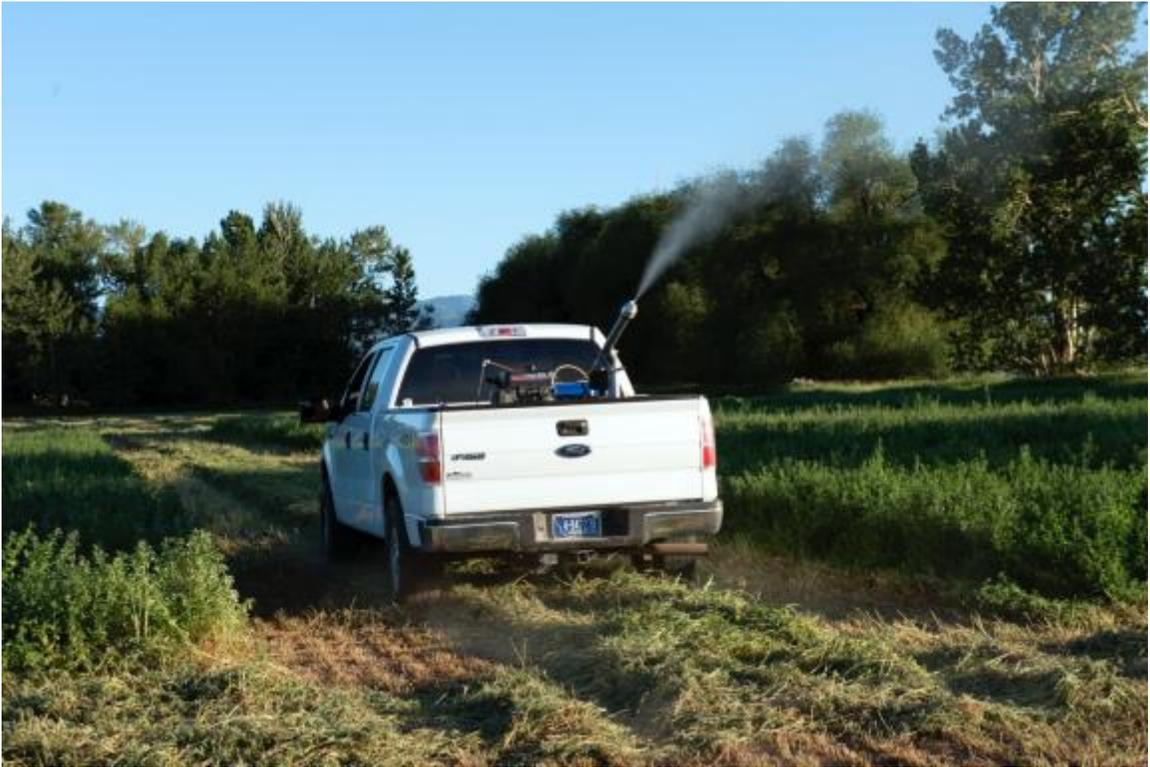
Figure 5. Ultra-low-volume applicator releasing a formulation over an alfalfa field.
