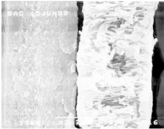
Fig. 4. SEM image of fouling layer. The fouling layer is on the left and membrane on the right.
