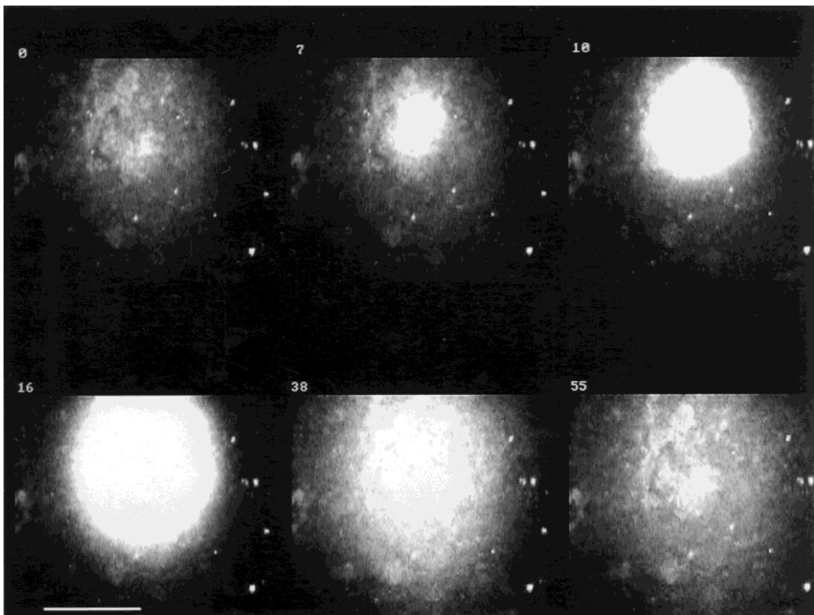
**Figure 3.** The expansion and dissipation of a fluorescent plume after a pulse injection of fluorescein dye monitored with confocal microscopy. The diffusion coefficient was calculated from the time taken for a concentration wavefront to reach a known distance from the origin. Images were taken at the indicated times (s) after injection. Scale bar = 250  $\mu\text{m}$ .
