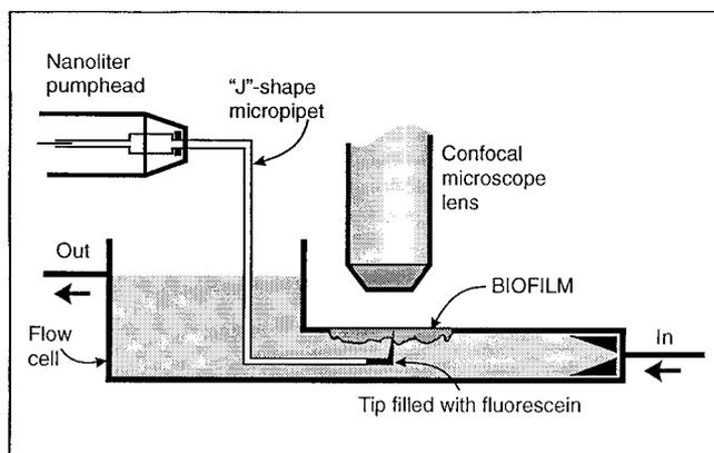
**Figure 1.** Schematic of the experimental set-up: pumphead with J-shaped micropipet, confocal microscope lens, flow cell, and observation window with biofilm.
