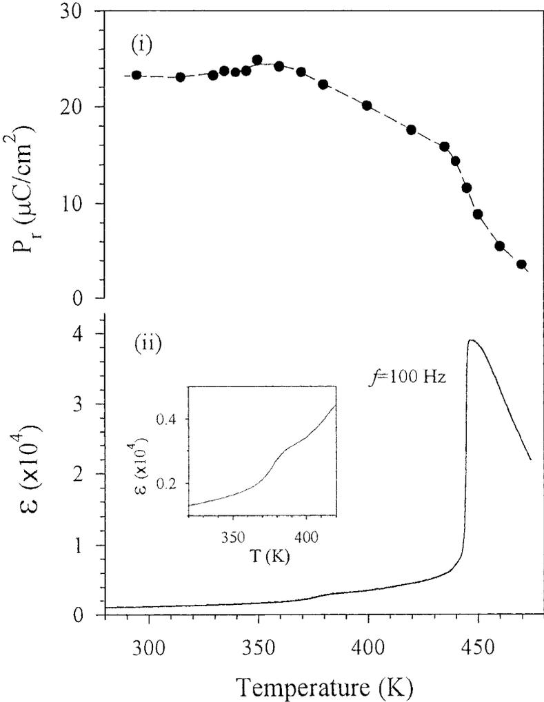
**Figure 2.** Temperature dependences of (i) remanent polarization  $P_r$  and (ii) dielectric permittivity  $\epsilon$ . The dashed lines are guides for the eye.
