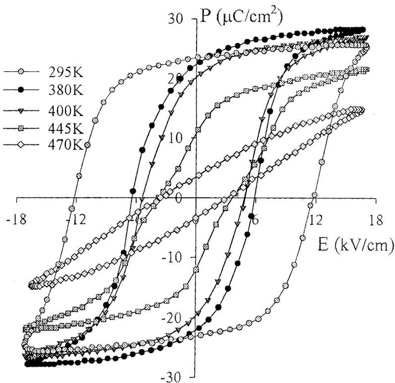
Figure 1. P-E hysteresis loops upon heating sequence.
