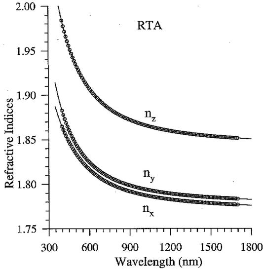
Fig. 3. Refractive indices ( $n_x$ ,  $n_y$ ,  $n_z$ ) of RTA. Solid lines are fits to the Cauchy equations with parameters given in Eq. (4).
