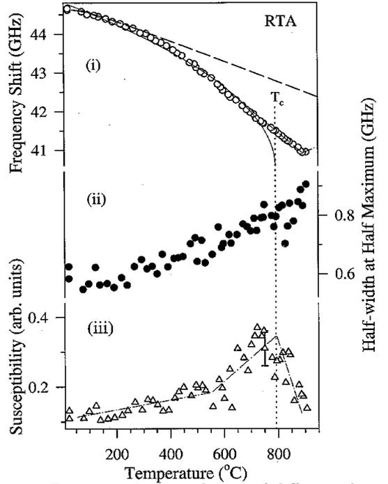
Fig. 2. Temperature dependences of different characteristics: (i) Brillouin shift (open circle), (ii) half-width (solid circle) and (iii) susceptibility constant (triangle). The dashed line is the Debye anharmonic calculation with parameters mentioned in the text. The solid line is a fit of the equation,  $\omega = a(T_c - T)^{1/2} + b$ . The dotted line indicates the ferroelectric phase transitions at  $T_c \sim 794$  °C. The dot-dashed lines are guides to the eye.
