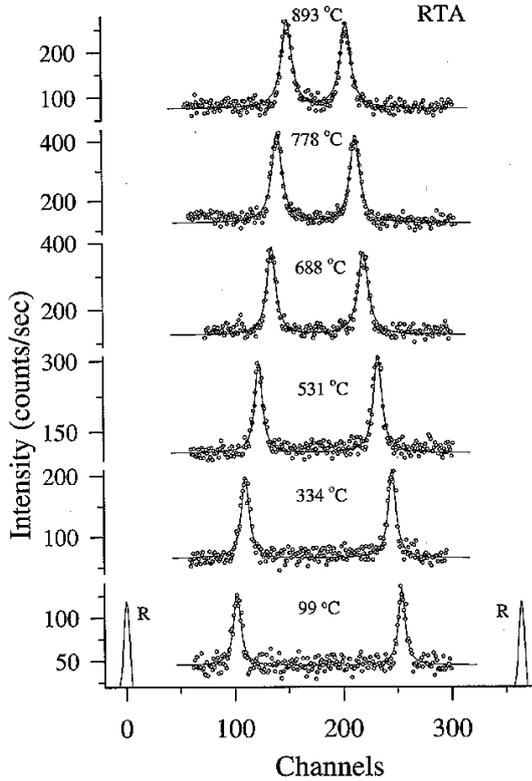
Fig. 1. Anti-Stokes and Stokes components of the LA[001] Brillouin spectra for RTA. The frequency interval (FSR) between the two Rayleigh (R) peaks is 25.79 GHz. The solid lines are fits of Eq. (1). Here, the rate of GHz/channel is 0.071.
