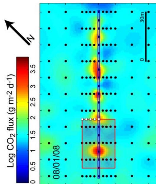
**Fig. 10** Map of log soil CO<sub>2</sub> flux, interpolated based on measurements made at the black dots [modified from Lewicki et al. 2009, (this volume)]. The blue rectangle represents the CO<sub>2</sub> injection well. The red rectangle marks the plant study area. White squares are soil CO<sub>2</sub> concentration probes. Note the two zones of high CO<sub>2</sub> flux at the east edge and in the center of the plant study area
