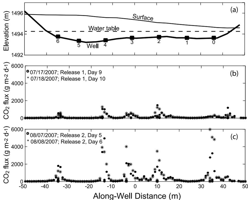
**Figure 1.** (a) Surface, horizontal well, and approximate water table elevation (water table depth only measured near packer 5). Black squares are packers numbered 0–6. Plots of  $F_{\text{CO}_2}$  measured along the surface well trace on (b) 17–18 July 2007 and (c) 7–8 August 2007. Distance = 0 m corresponds to grid origin shown in Figure 2.
