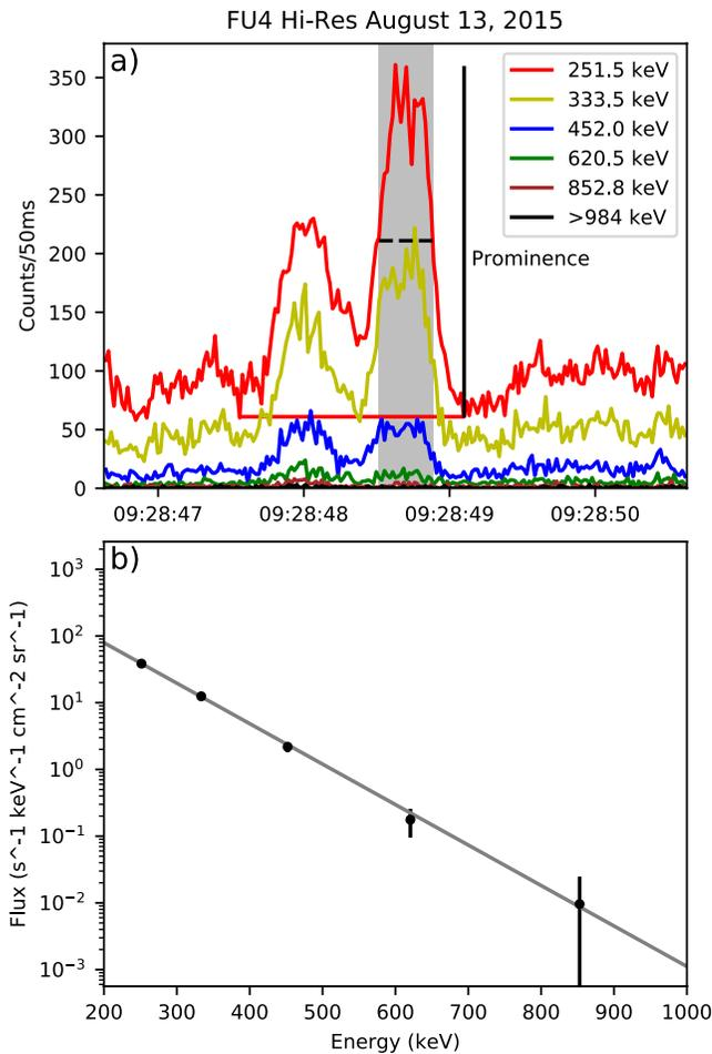
**Figure 2.** Example microburst and fit energy spectrum. Panel (a) shows the FIREBIRD time series data. The shaded gray area represents the time range each energy in the microburst was integrated over, calculated at half prominence in the lowest energy channel as shown with the dashed horizontal black line. The horizontal red line represents the background levels for the 251.5-keV channel. Panel (b) shows the GEANT-determined flux in each energy channel and best-fit e-folding function.
