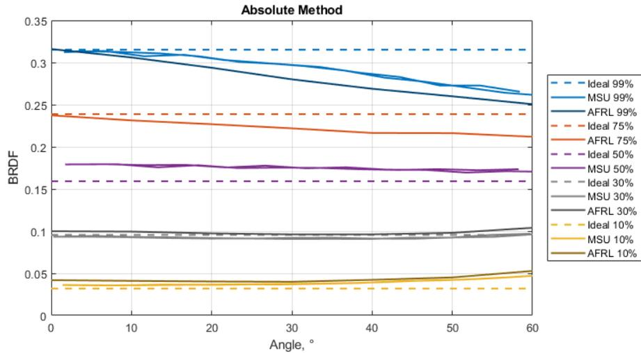
**Figure 2.** Summary of Spectralon monostatic BRDF measurements as compared to the ideal for a Lambertian surface of each panels' nominal reflectance, using the absolute method of BRDF calculation.
