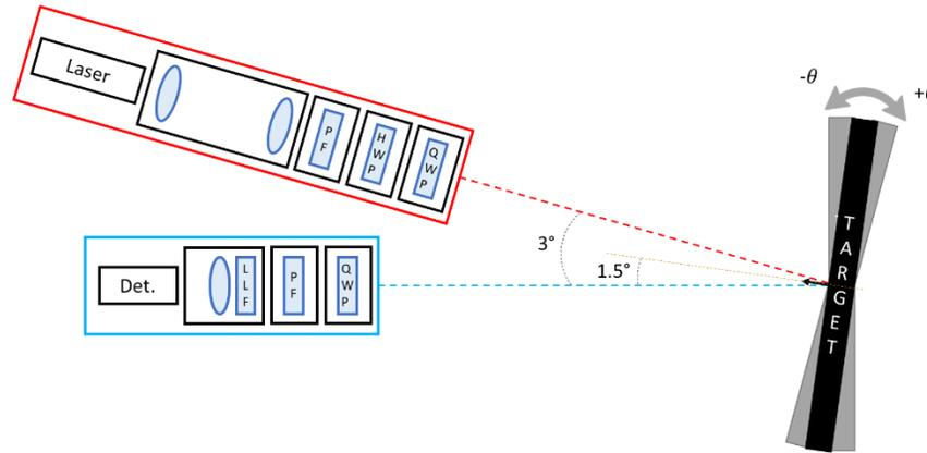
**Figure 1.** Exaggerated angular geometry of the Mueller lidar test-bed. A  $0^\circ$  incidence/viewing angle is defined when the surface normal of the target is  $1.5^\circ$  from the optical paths of both the transmitter and the receiver.
