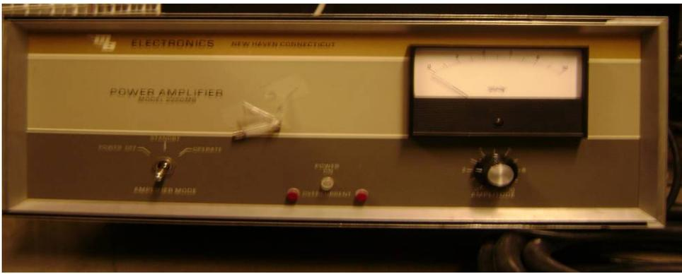
Figure 7: The power amplifier for create vibration
