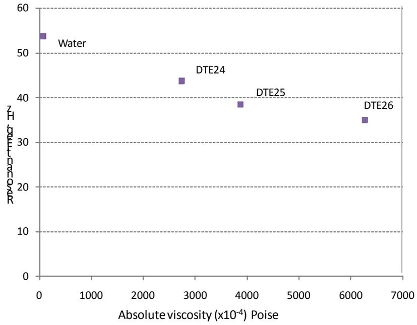
Figure 16: Resonant Frequency variation with viscosity (Configuration B).
