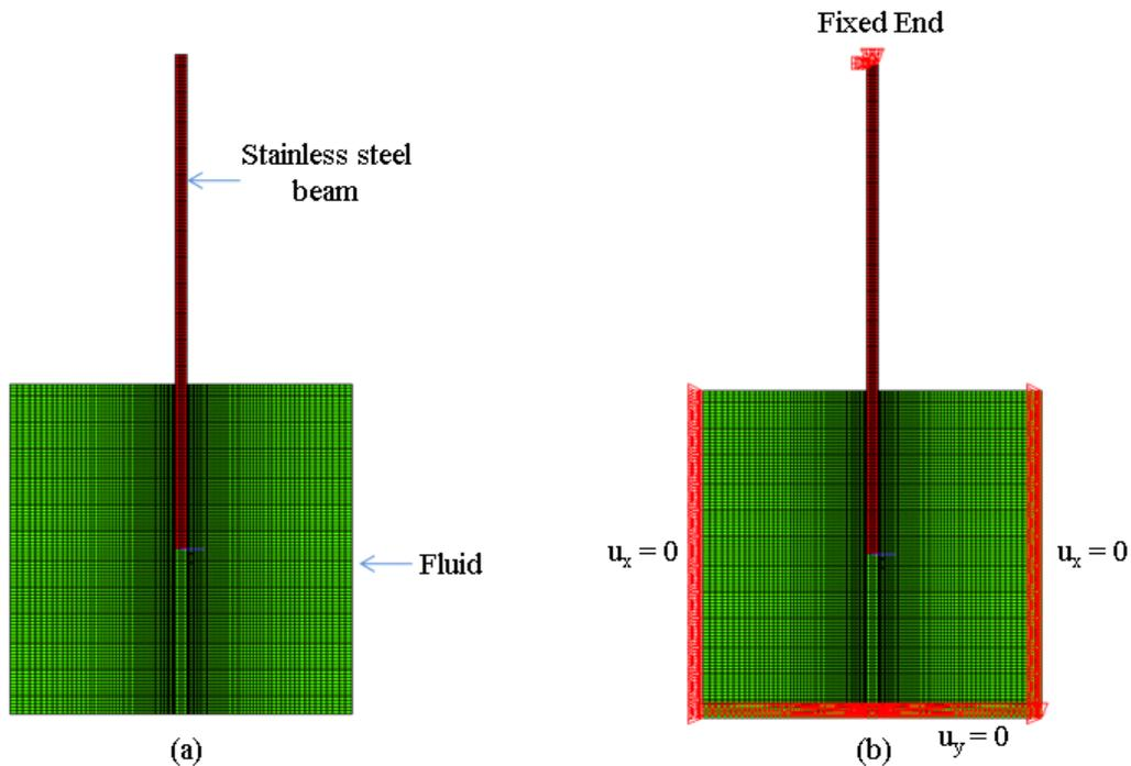
Figure 25: FE model of cantilever beam partially submerged under fluid.
