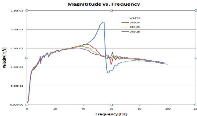
Figure 15: 1<sup>st</sup> Frequency response curve in different fluid media (Configuration B).
