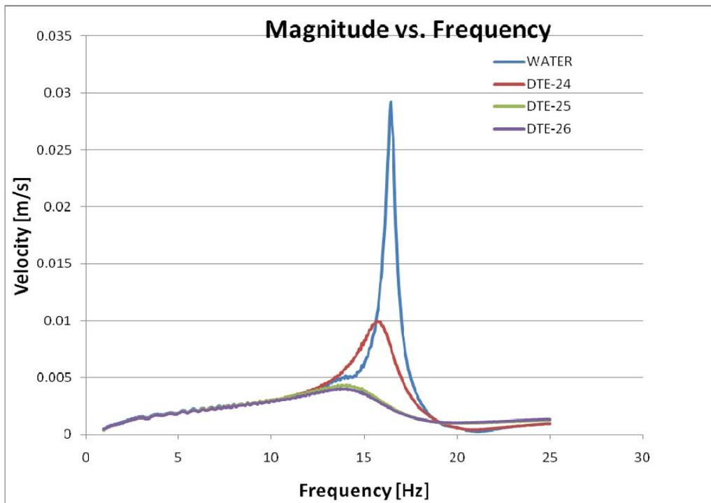
Figure 11: Frequency response curve in different fluid media (Configuration A).
