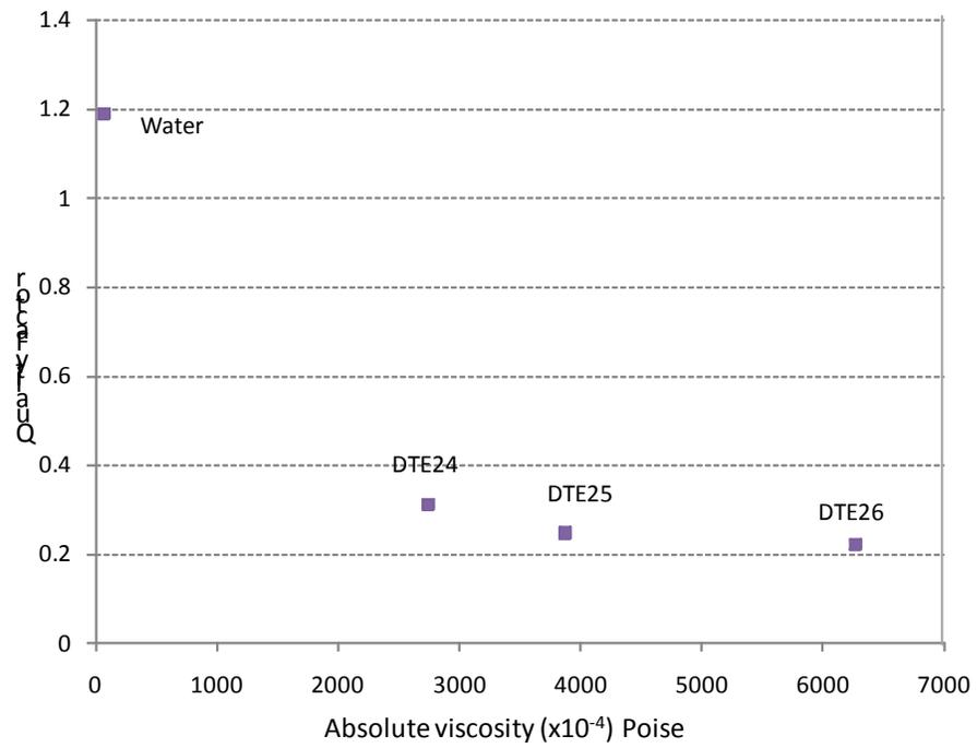
Figure 17: Quality factor (Q) variation with viscosity (Configuration B).
