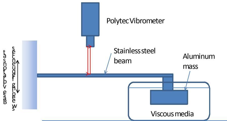
Figure 1: End mass oscillates in viscous fluid (Configuration A).
