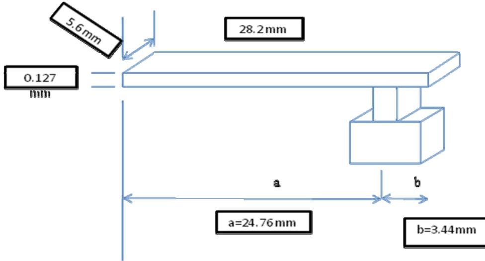
Figure 18: Dimensions of the beam with load ( configuration A).
