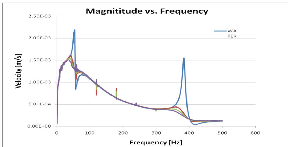
Figure 14: 1<sup>st</sup> and 2<sup>nd</sup> Frequency response curves in different fluid media (Configuration B).
