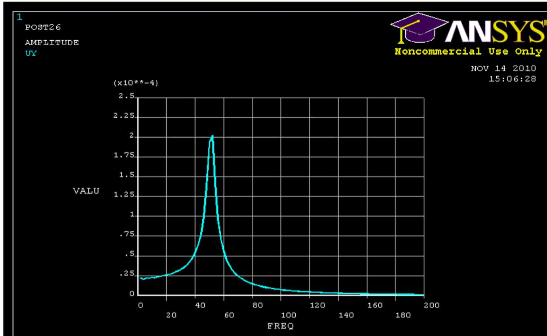
Figure 28: Result found by harmonic solution for water.
