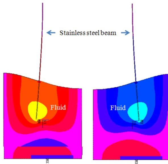
Figure 26: Mode shape for the 1<sup>st</sup> resonant vibration in transverse direction.
