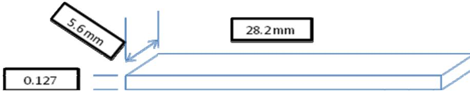
Figure 19: Dimensions of the beam with load (configuration B).
