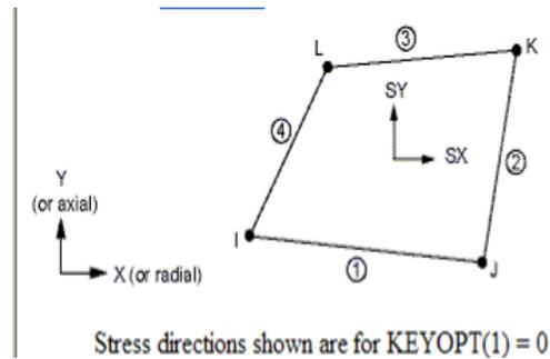
Figure 22: PLANE 42 stress output.
