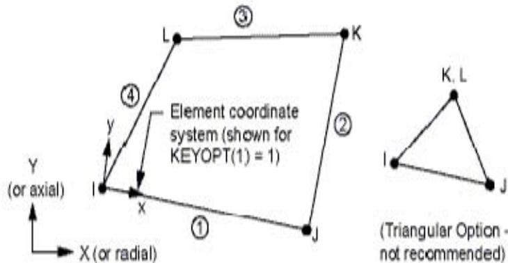
Figure 21: PLANE42 Geometry.
