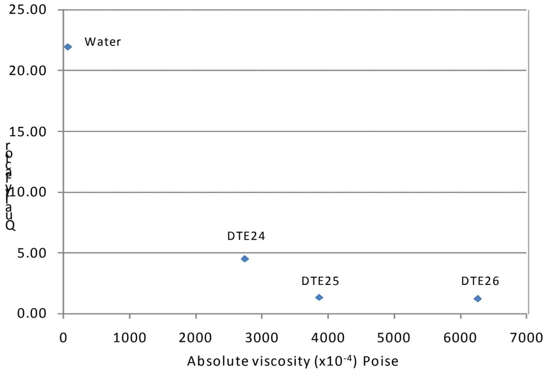
Figure 13: Quality factor (Q) variation with viscosity (Configuration A).
