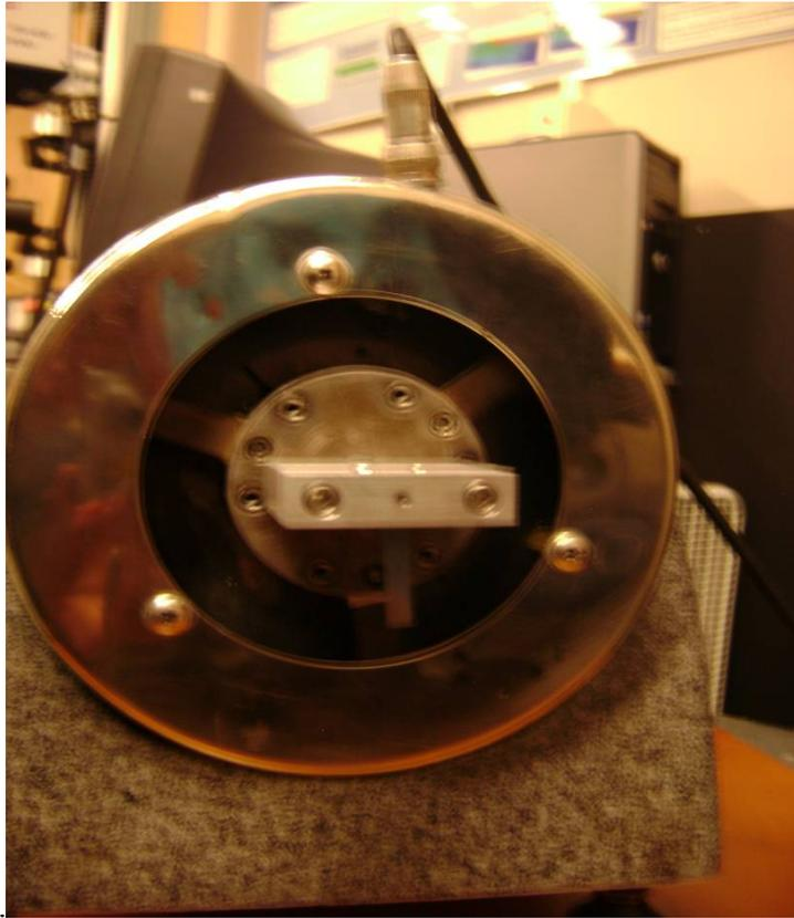
Figure 8: Shaker with connecting cord of amplifier and beam holder.
