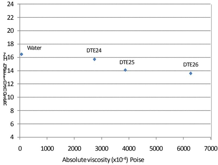
Figure 12: Resonant Frequency variation with viscosity (Configuration A).
