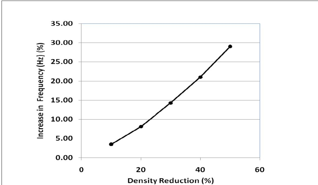
Figure 27: Increase of frequency by the decrease of density of viscous fluids.
