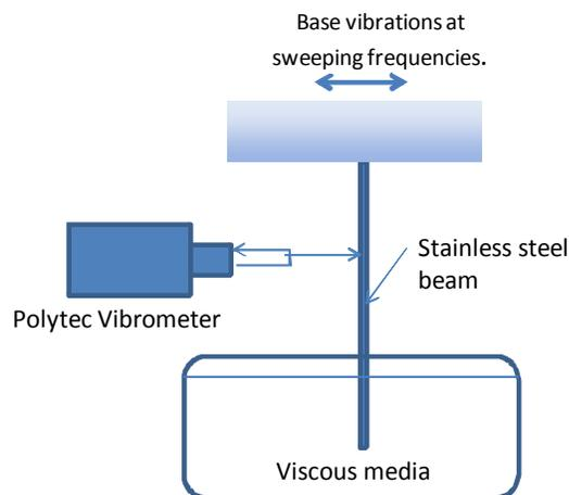
Figure 2: Beam end oscillates in viscous fluid (Configuration B).
