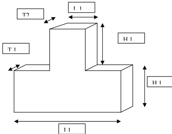
Figure 9: The T shaped Aluminum mass of configuration A.
