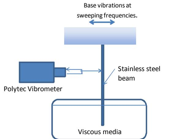
Figure 20: Experimental setup to predict modal response of cantilever beam.
