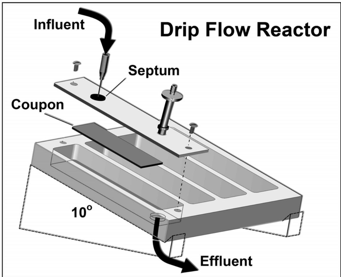
Figure 2.3. Drip flow biofilm growth setup.
