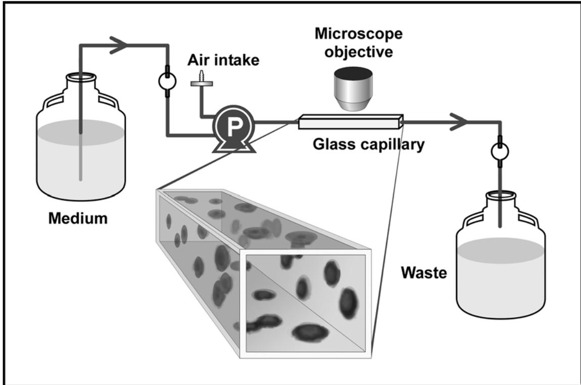
Figure 2.2. Capillary biofilm growth setup.
