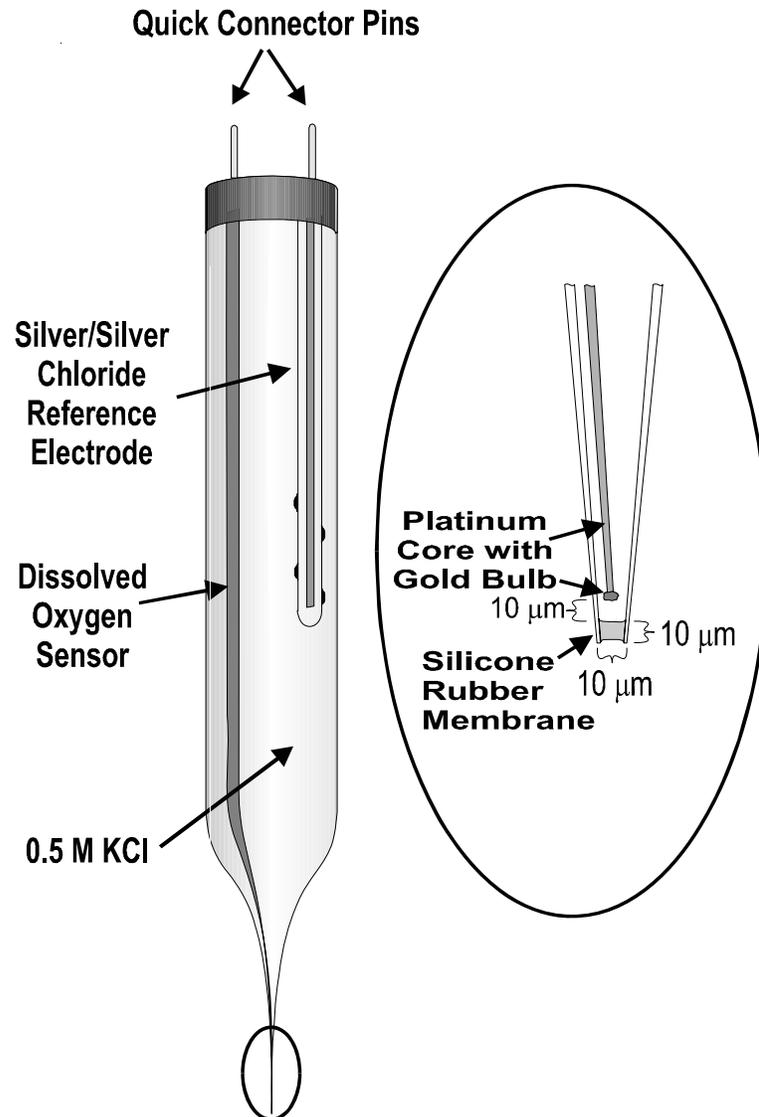
Figure 2.4. Dissolved oxygen microelectrode.
