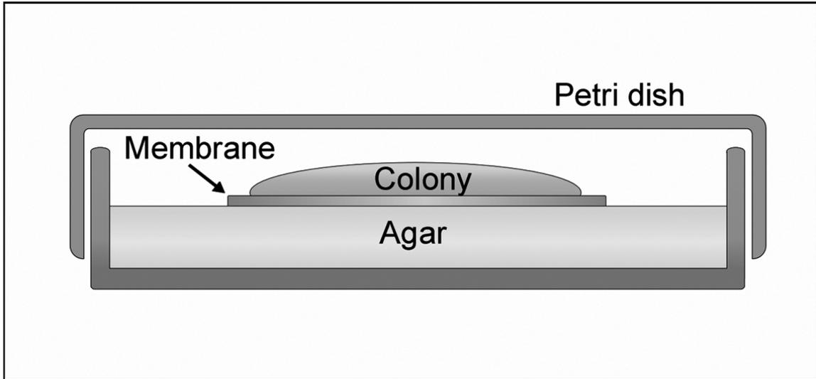
Figure 2.1. Colony biofilm growth setup.
