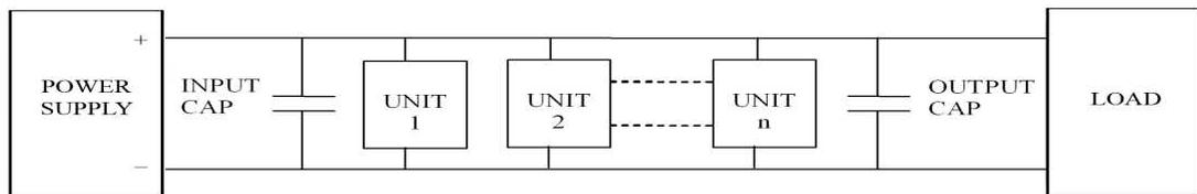
Figure 20. Interleaving of DC-DC Converters
