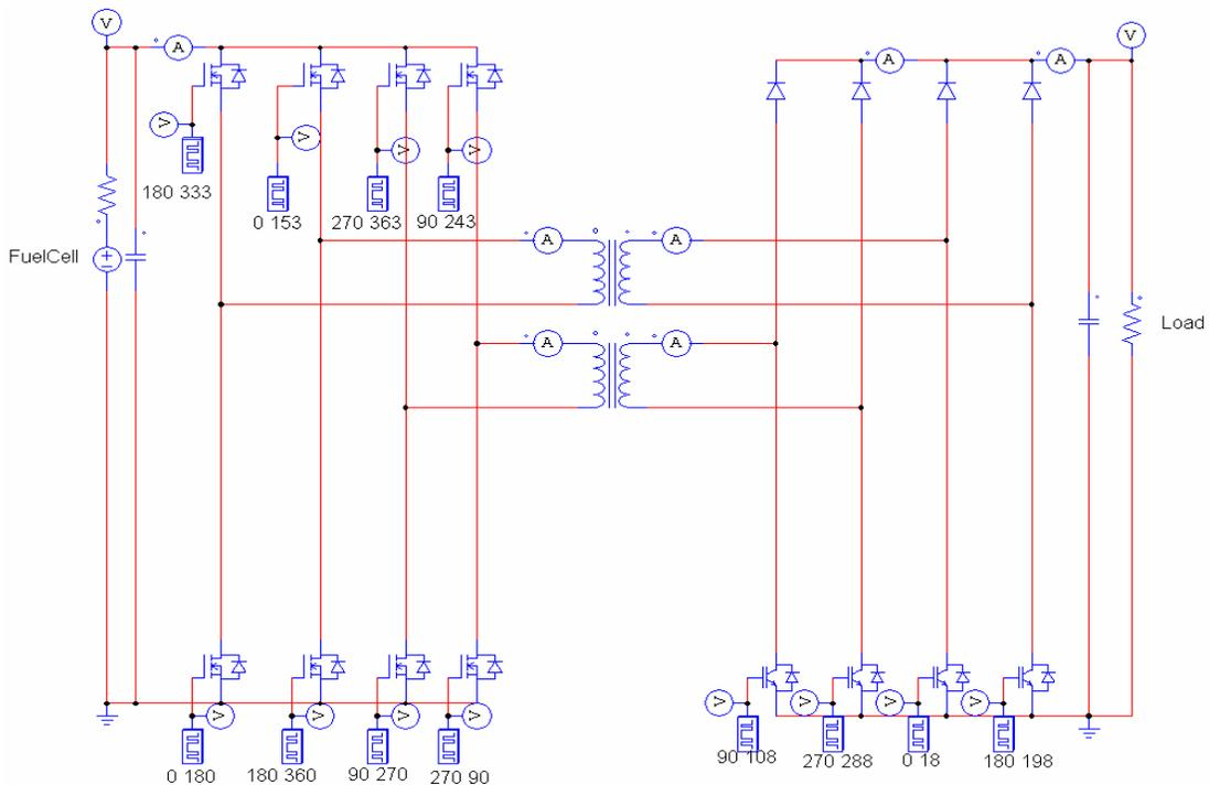
Figure 21. Simulation Schematic of Two 550W Interleaved Units of the Proposed Converter
