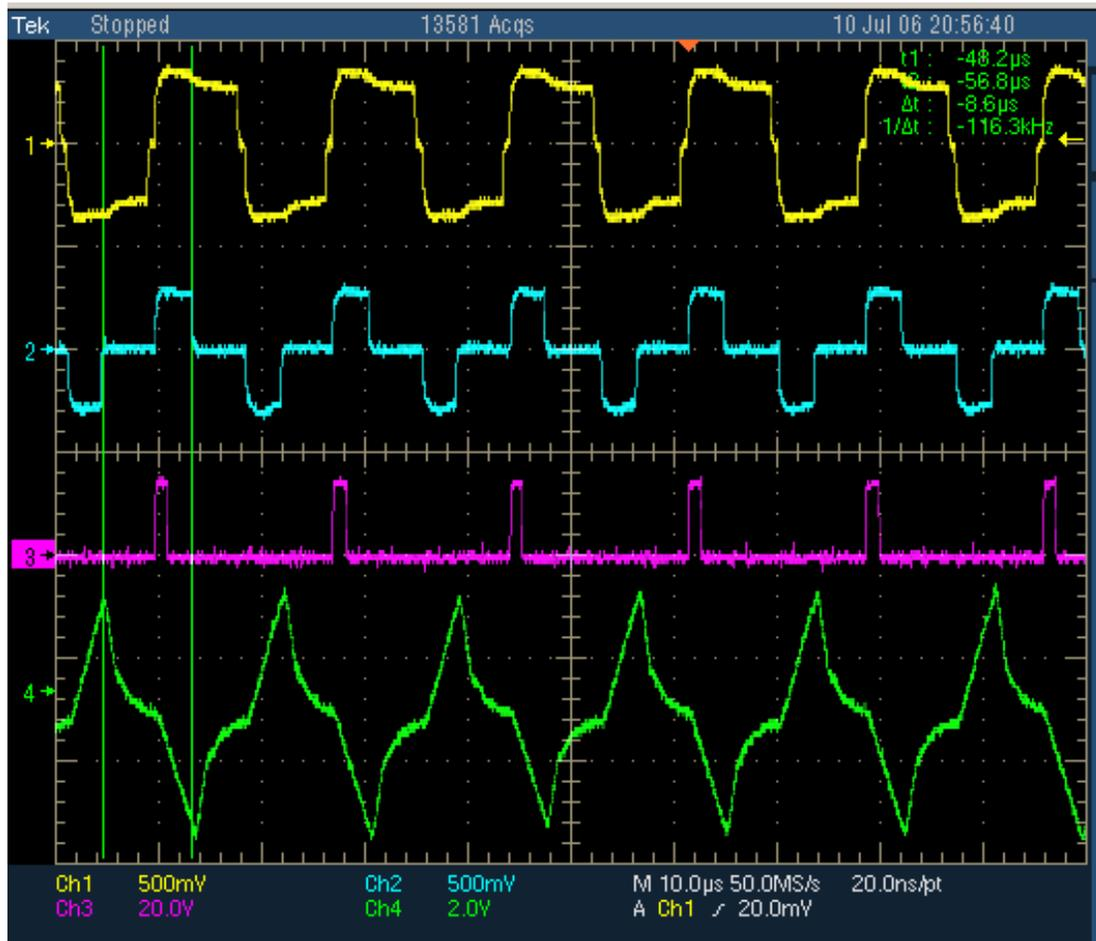
Figure 29. Synchronized, Isolated PWM Control Signals and Transformer Current
