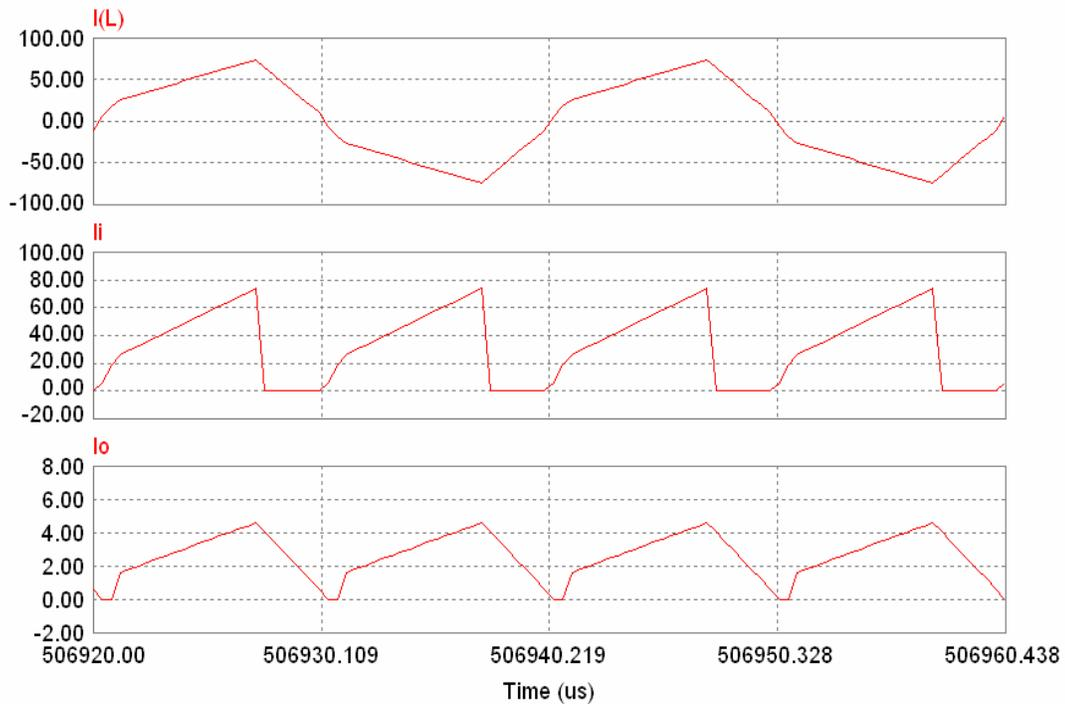
Figure 23. Simulation Results for Stand Alone Single 1.1kW Unit. From Top to Bottom: Current through the Isolation Ttransformer, Input Current and Output Current
