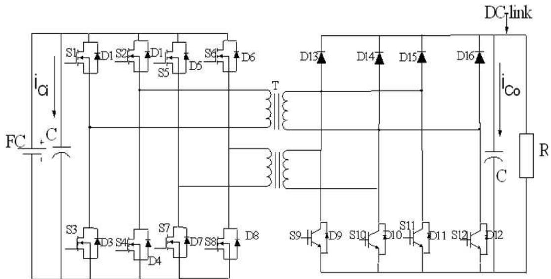
Figure 24. Schematic of Two Interleaved Units of Proposed Converter
