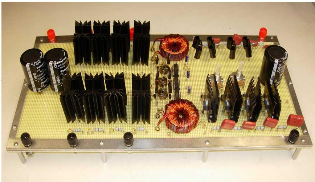
Figure 25. 1.1kW Interleaved-Units Prototype Breadboard
