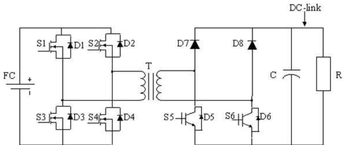
Figure 5. Topology of the Proposed DC/DC Converter
