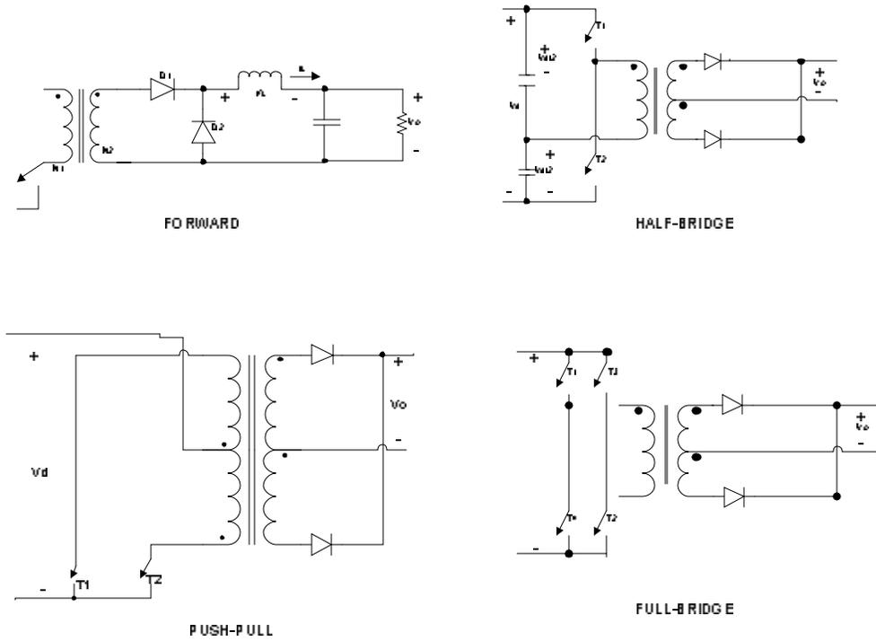
Figure 4. Conventional Isolated DC-DC Converters
