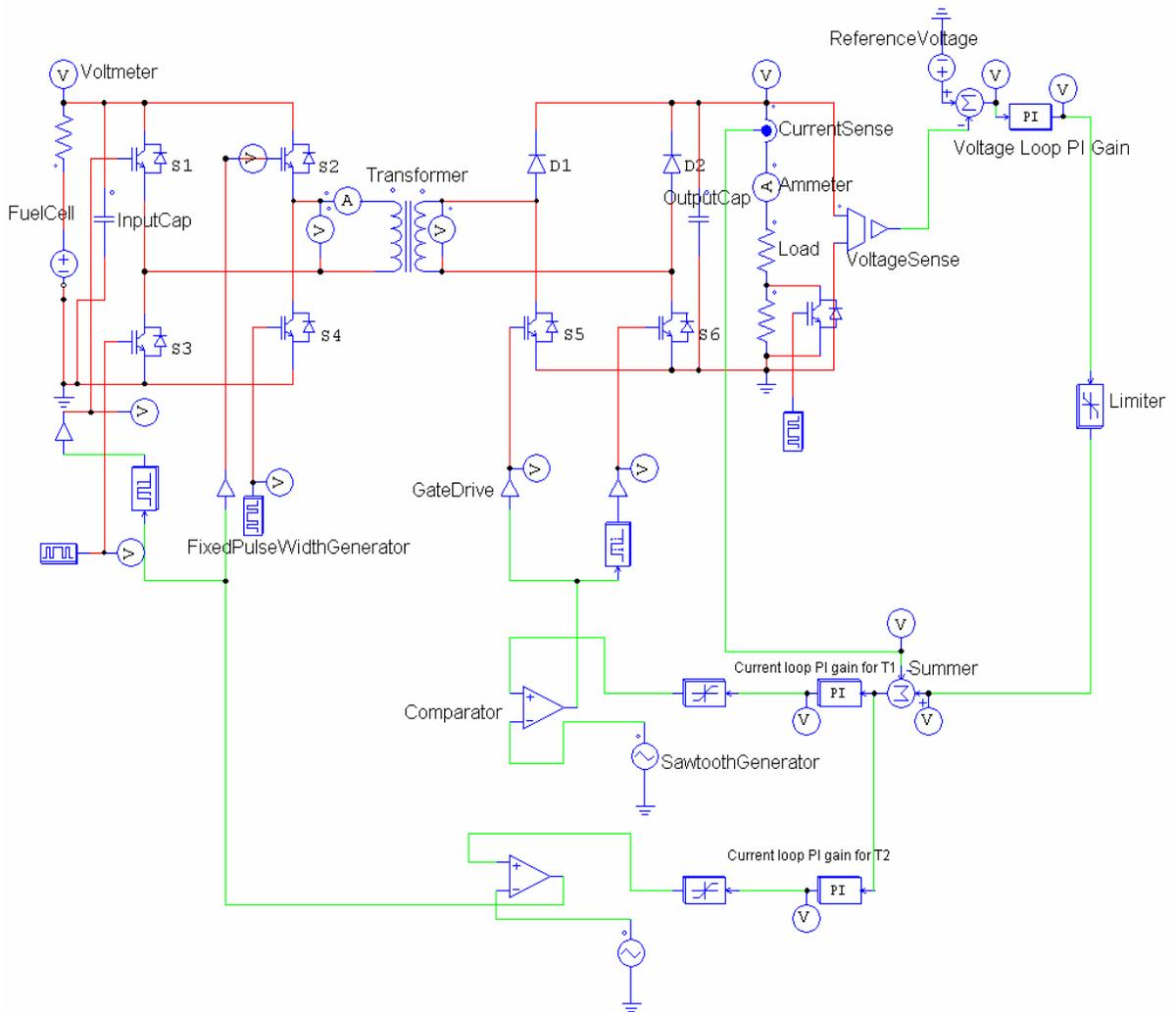
Figure 12. Simulation Schematic of the Proposed Converter
