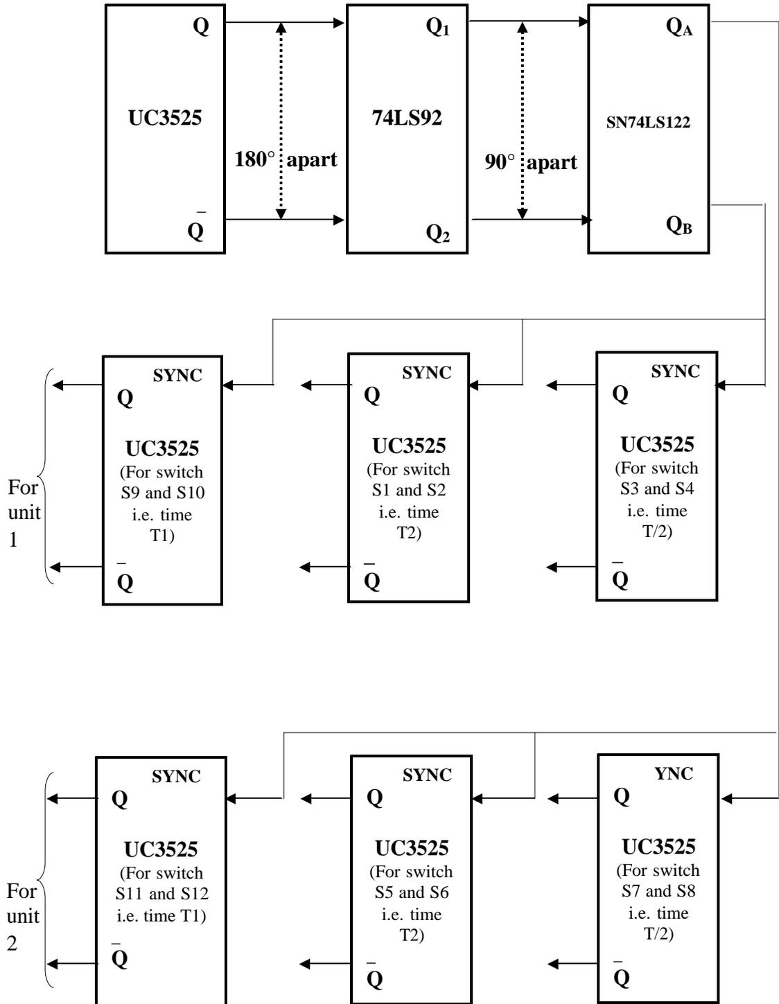
Figure 27. Block Diagram of 90 Degrees Phase Shifting of PWM Signals for the Interleaved Units
