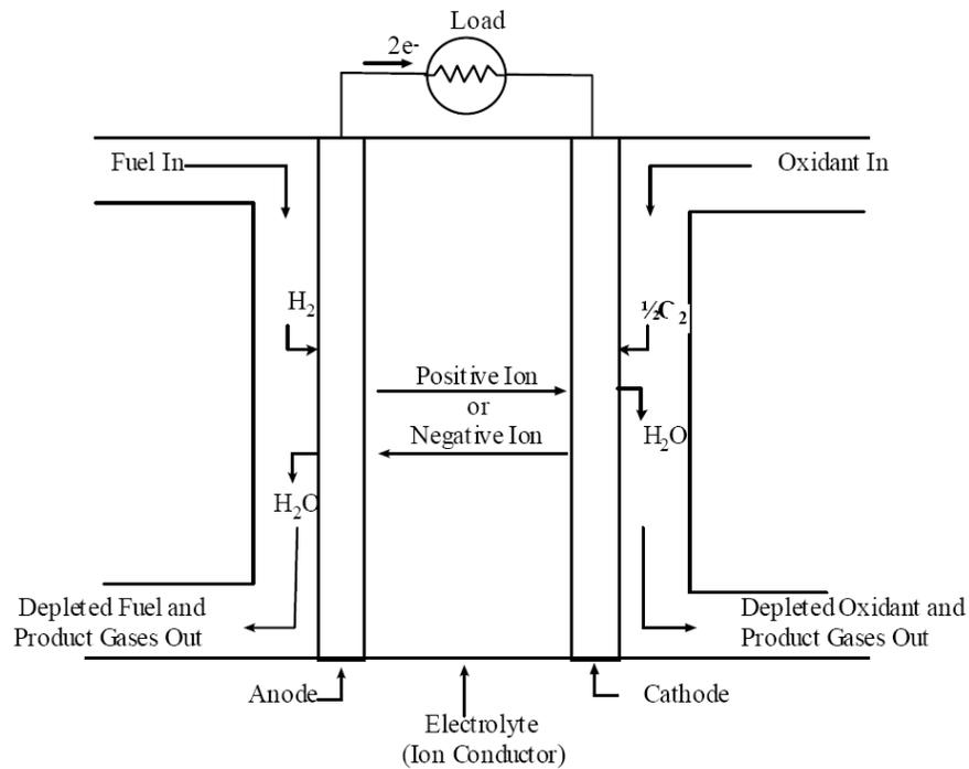
Figure 1. Schematic of a Fuel Cell
