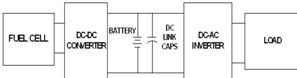
Figure 3. Typical Fuel Cell Powered Residential Power Generation System
