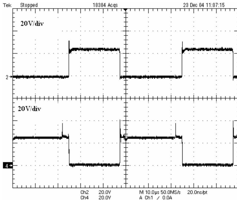
Fig. 17. From Top to Bottom: Experimental Recorded Voltage Across the Upper MOSFET (20V/div) and Across the Lower MOSFET (20V/div) of the Same Leg in the Primary Side with a Time Base of 10µs/div
