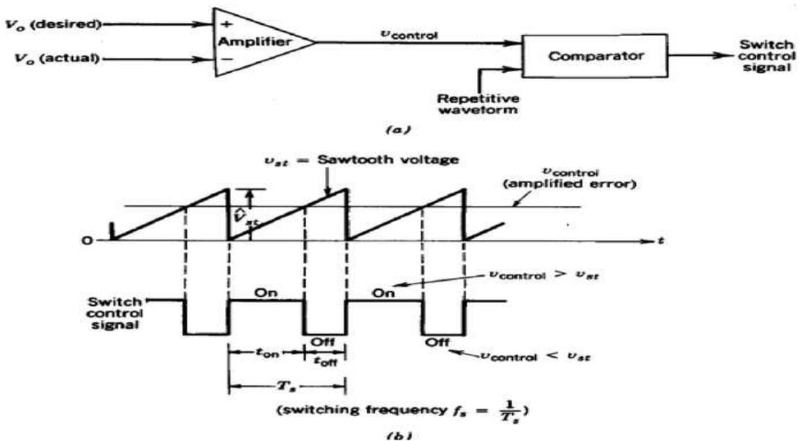
Figure 9. Pulse-Width Modulator: (a) Block Diagram, (b) Comparator Signals
