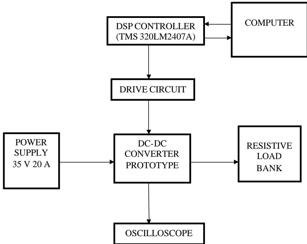
Figure 15. Laboratory Setup Schematic of 350W Prototype
