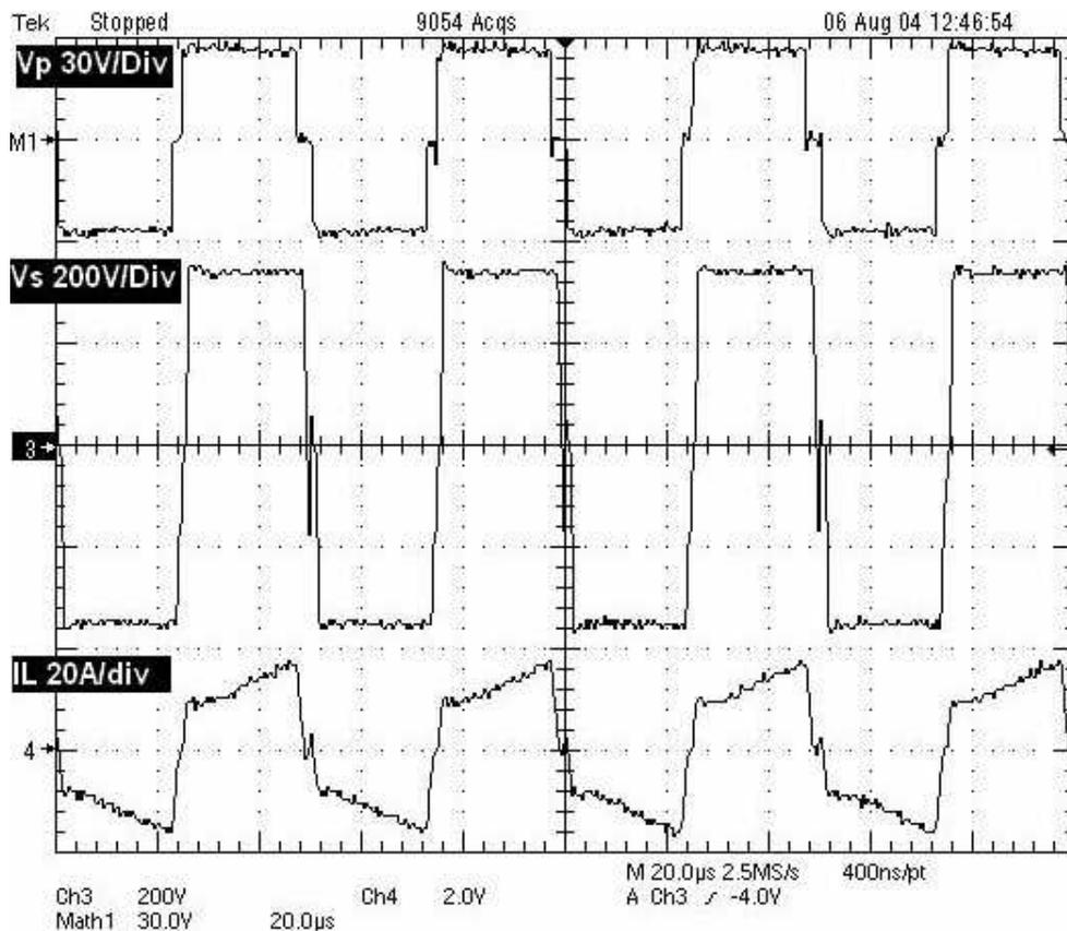
Figure 16. From Top to Bottom: Experimental Recorded Voltage of the Primary Side of the Transformer (30V/div), Voltage of the Secondary Side of the Transformer (200V/div), and Current of the Primary Side of the Transformer (20A/div), with a Time Base of 20µs/div
