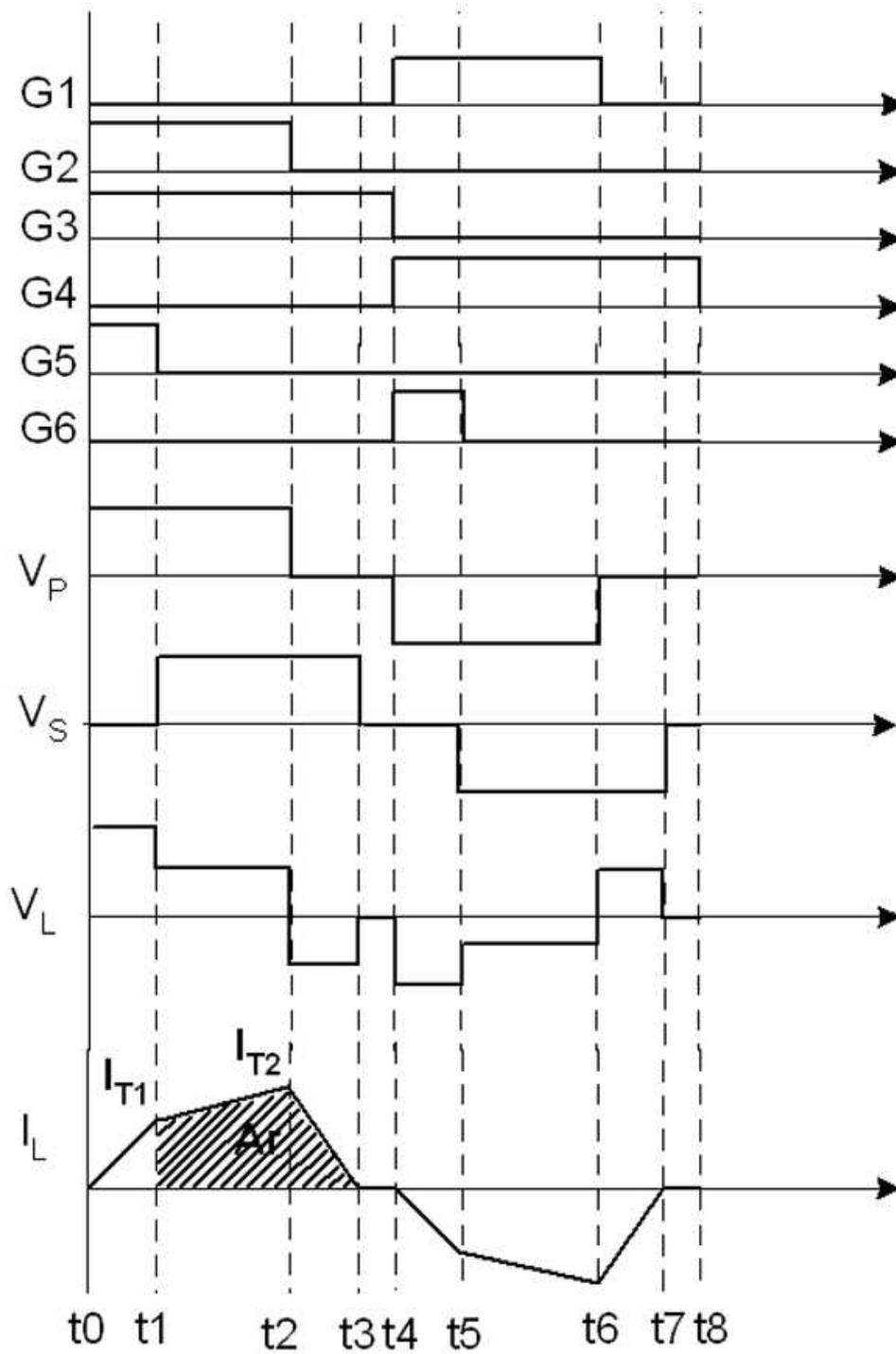
Figure 7. Waveforms of Key Components of the Converter in One Complete Cycle
