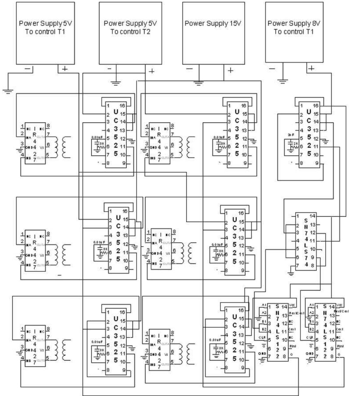
Figure 28. Schematic of 90 Degrees Phase Shifting of PWM Signals for the Interleaved Units
