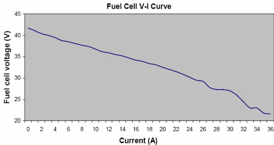
Figure 2. Typical Fuel Cell Voltage / Current Characteristics [8]
