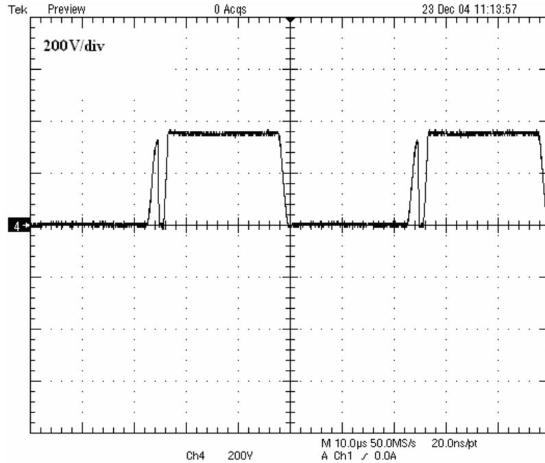
Figure 18. Experimental Recorded Voltage Across the MOSFET (200V/div) in the Secondary Side with a Time Base of 10µs/div
