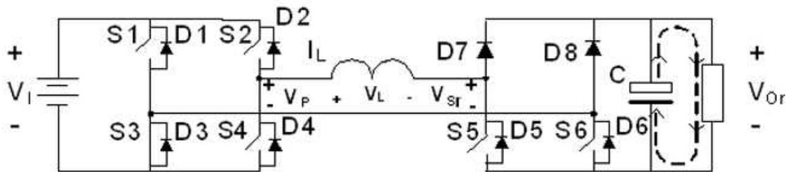
Figure 6. Transformer Primary Side Referred Equivalent Circuits of the Converter During Different Time Periods in the First Half Cycle
