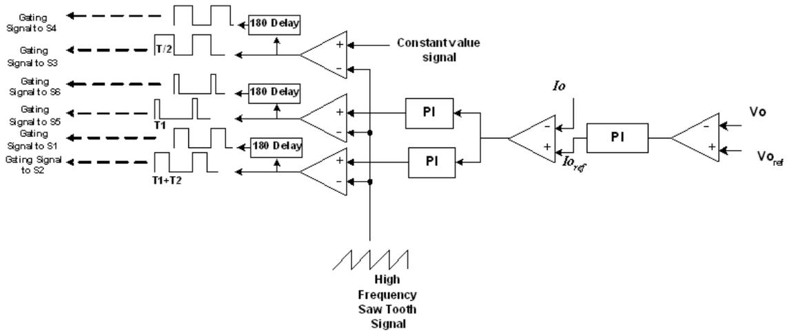
Figure 8. Control Scheme of Proposed Converter
