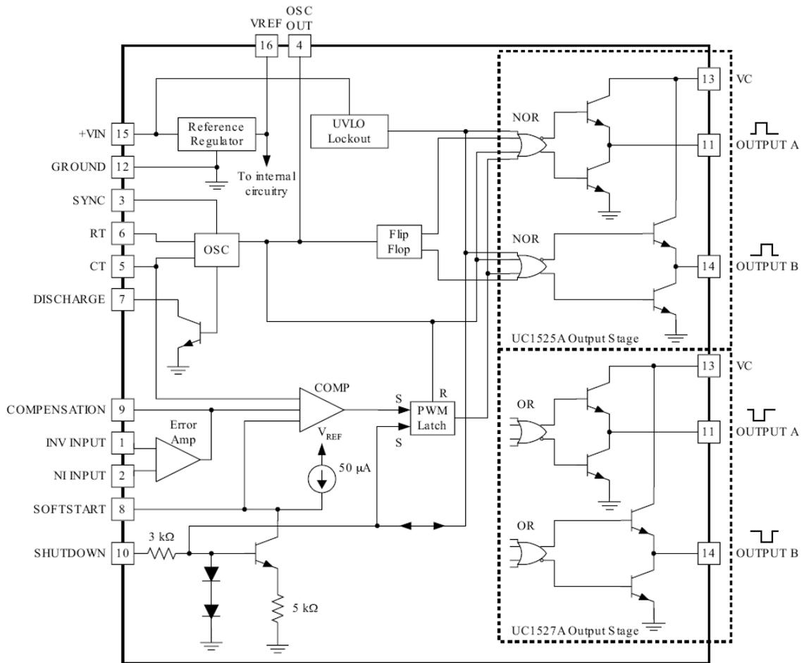
Figure 26. Pin Out and Internal Logic Diagram of UC3525
