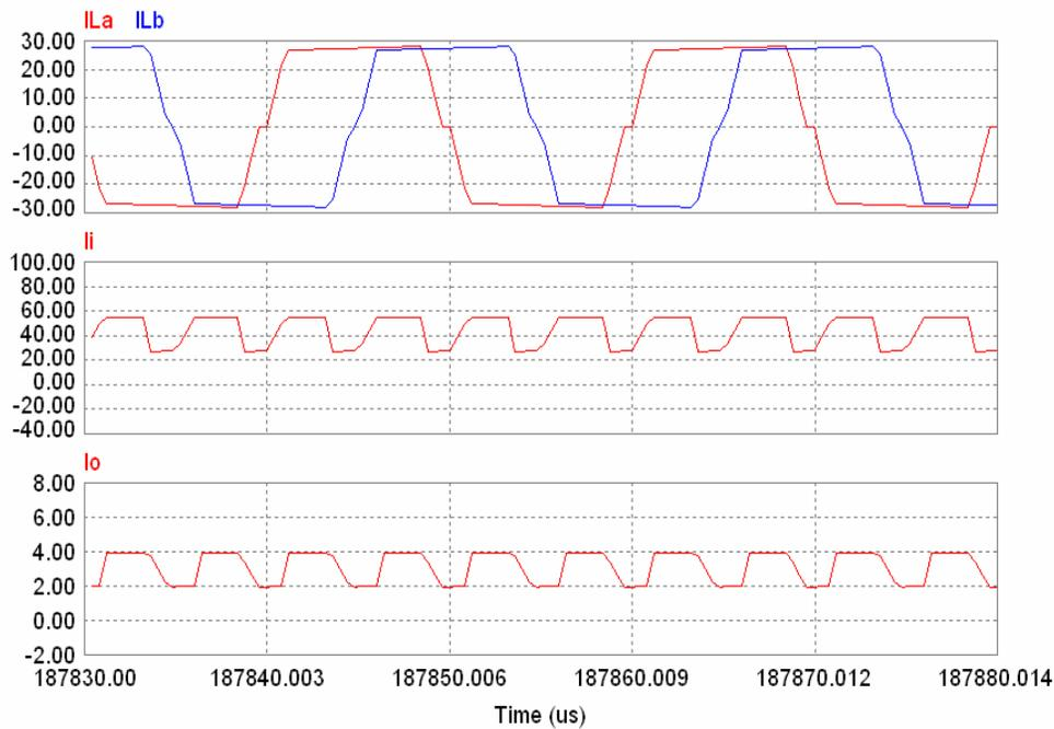
Figure 22. Simulation Results for Two Interleaved 550W Units. From Top to Bottom: Current through the Two Isolation Transformers, Input Current and Output Current
