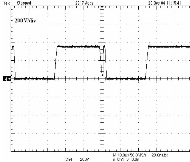
Figure 19. Experimental Recorded Voltage Across the Diode (200V/div) in the Secondary Side with a Time Base of 10µs/div
