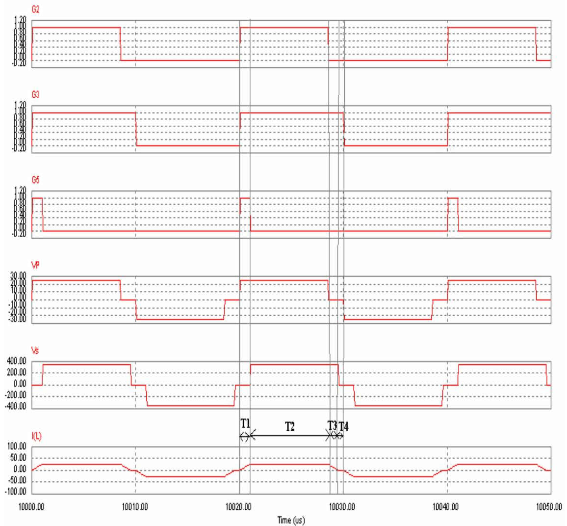
Figure 13. From Top to Bottom Open Loop Simulation Results of Gating Signal of Switch S2, Gating Signal of Switch S3, Gating Signal of Switch S5, Primary Side Voltage, Secondary Side Voltage, and Transformer Primary Current
