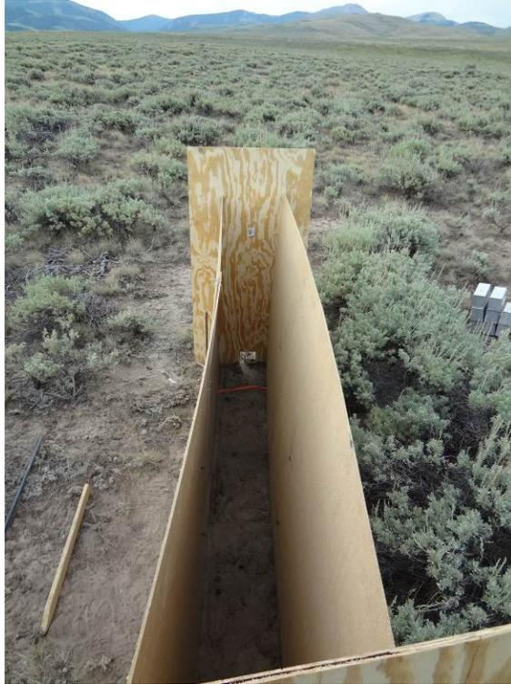
Figure 3.2. Track and the H2 Zoom unit used to record the noise made by deer mice moving through vegetation, shown in a cheatgrass-dominated site, central Montana, summer 2013.
