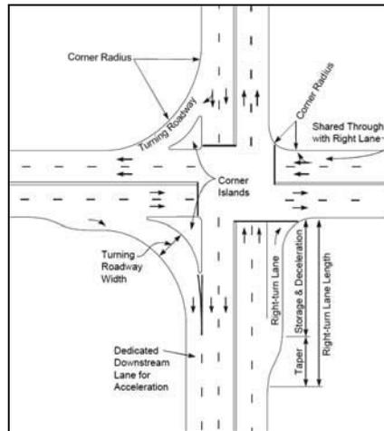
Fig. 1 - Right turning lane design elements [2]
