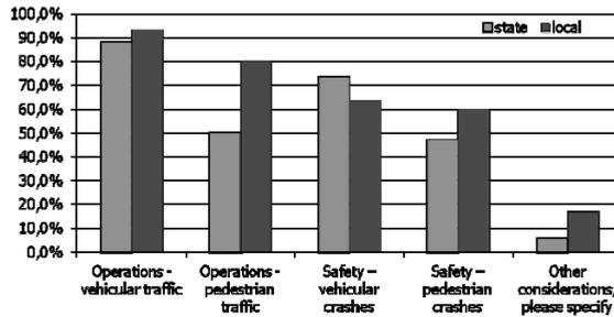
Fig. 5 - Considerations for traffic control device selection at CRTL
