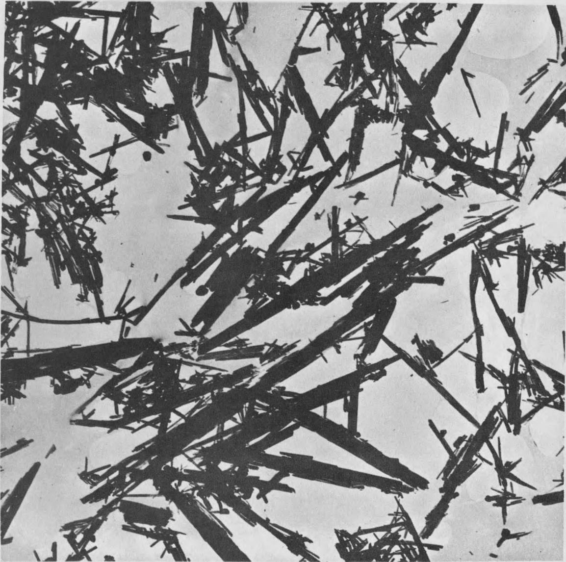
Figure 3 Electron Micrograph of  $\text{MnO}_2$  - 32,000X
