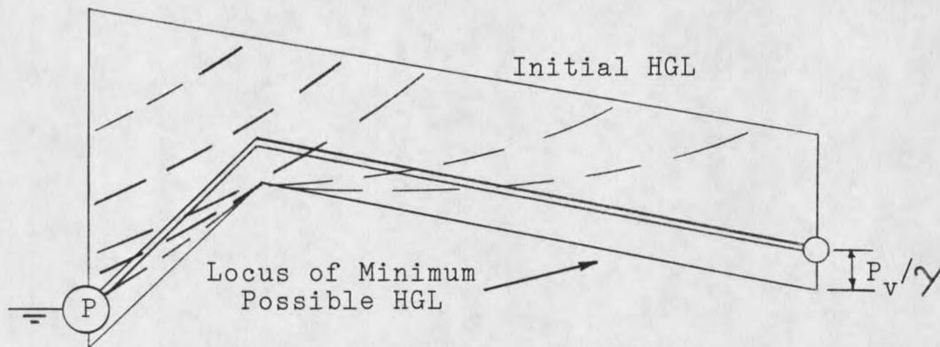
Figure 2. Progression of HGL during pump failure.
