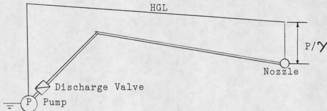
Figure 1. Schematic of typical sprinkler irrigation system.
