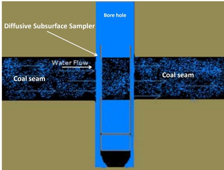
Figure 2: Sampling strategy used in this study: Schematic outlining the deployment of the DSM in CBM boreholes/wells. Sterile coal from the Decker Coal Mine (Powder River Basin) was loaded into the sampler and allowed to inoculate for three months. Upon retrieval the DSM closes to avoid contamination. At the surface slurry contained within the DSM was used to inoculate media and for community analysis.
