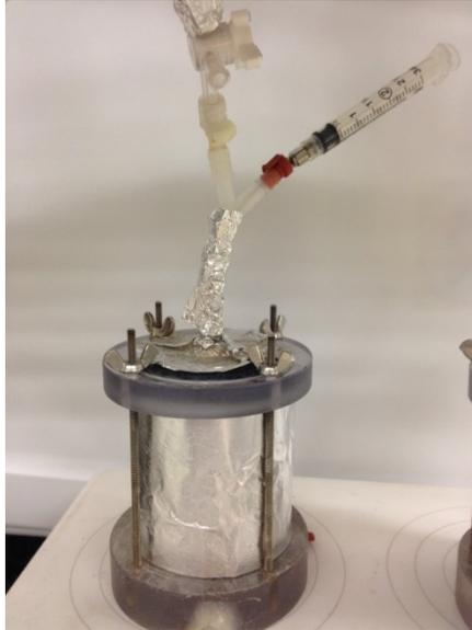
Figure 2: Packed bed reactor with "Y" in effluent line for sampling.
