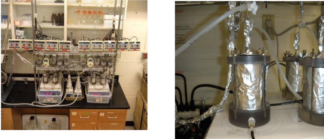
Figure 1: An overview of the packed bed reactor set up is shown on the left. A close up of a single packed bed reactor is shown on the right.
