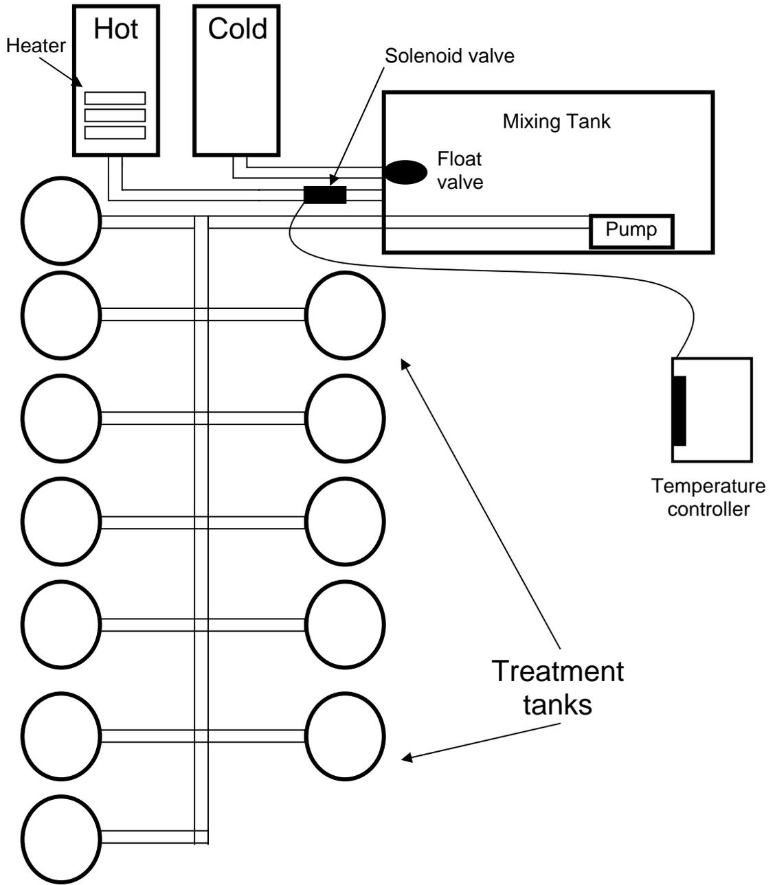
Figure 2. Schematic of laboratory design with hot and cold water inputs, mixing tank, solenoid and float valves, temperature controller, and treatment tanks.
