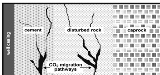
**Figure 1.** Schematic showing potential CO<sub>2</sub> leakage pathways in disturbed rock, cement and along well casing. This schematic represents the cement layer and disturbed rock at a location where the well passes through the cap rock, above the reservoir.
