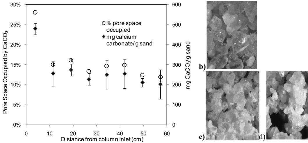
**Figure 3.** (a) Volume fraction of calcium carbonate-occupied pore space and CaCO<sub>3</sub> concentrations over the distance of the column. Stereoscopic analysis of (b) clean sand (control) and biofilm-calcium carbonate deposits (c - first 7.6 cm of column) and (d - last 7.6 cm of column) reveal significant calcium carbonate deposits.
