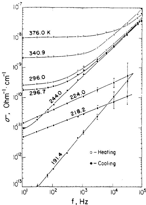
Fig. 4. Frequency dependences of the a.c. conductivity for KADP 0.6.
