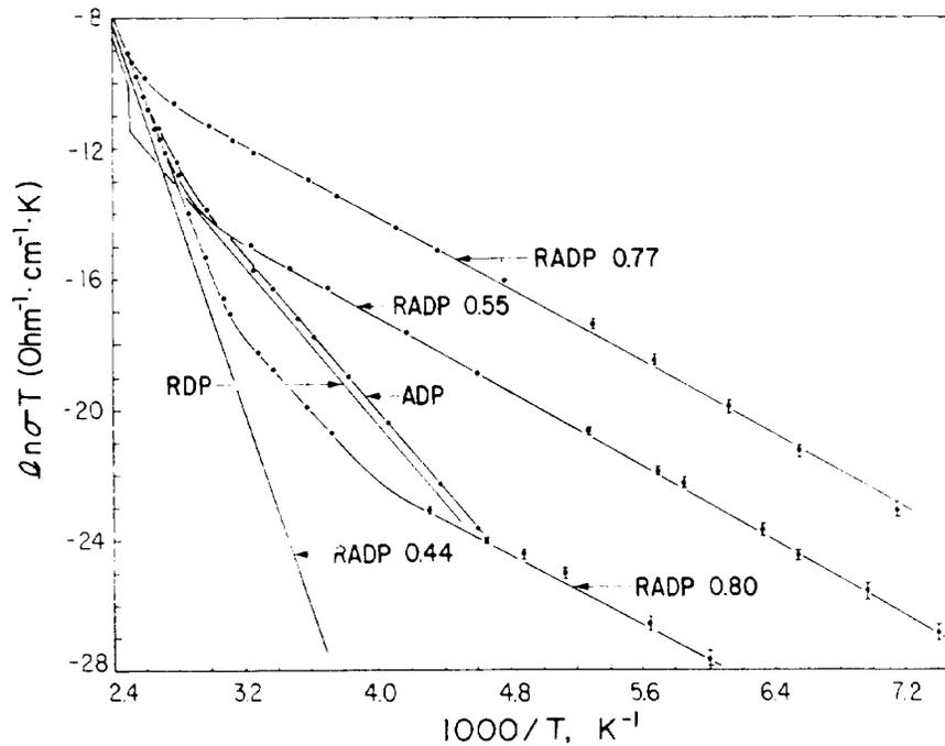
Fig. 2. Arrhenius plots of the d.c. bulk conductivity for different crystals of RADP, RDP and ADP. The RADP 0.44 results are from ref. [9].
