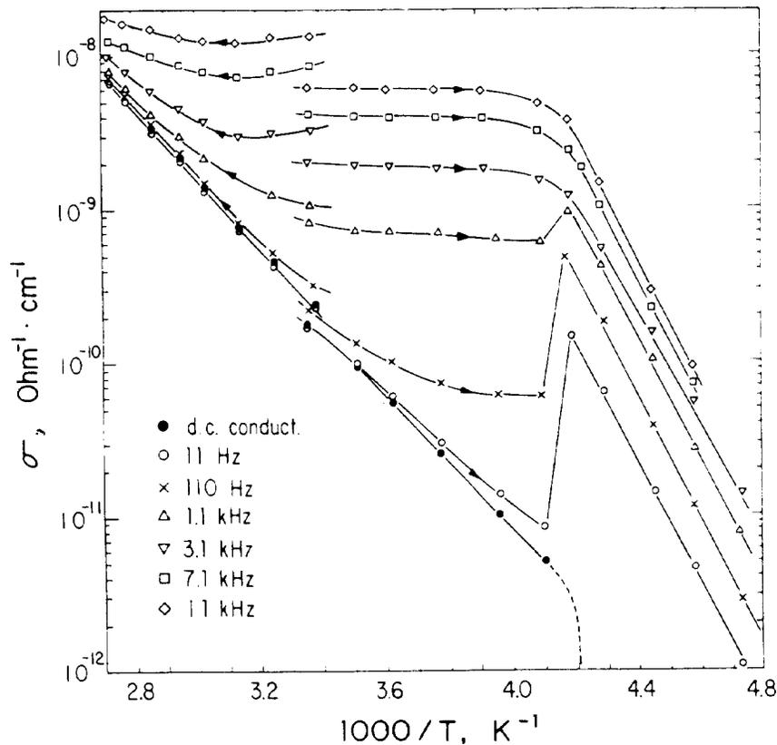
Fig. 3. Arrhenius plots of the d.c. bulk conductivity and a.c. conductivity for KADP 0.6.
