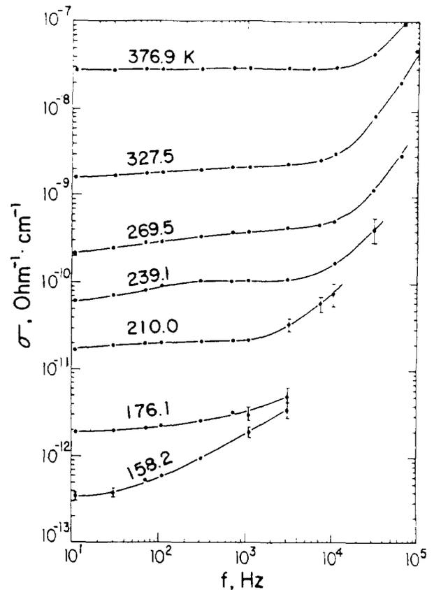
Fig. 5. Frequency dependences of the a.c. conductivity for RADP 0.5.
