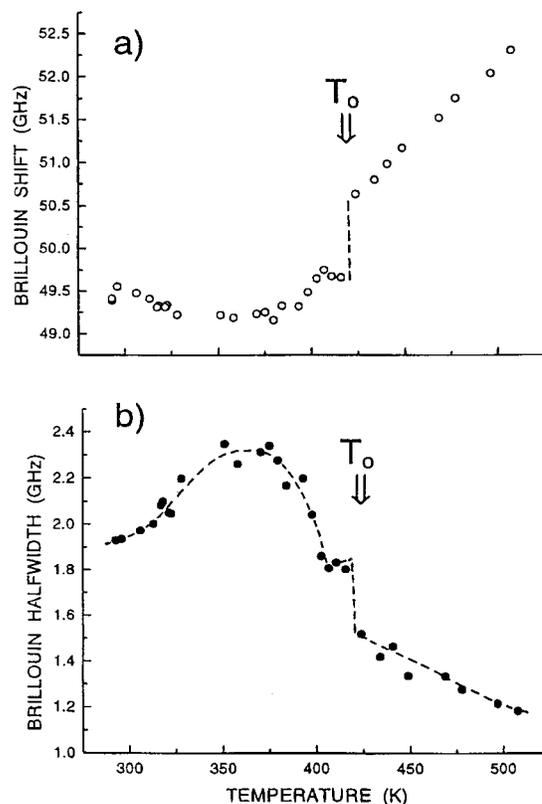
FIG. 2. The temperature dependence of the Brillouin shift (a) and the width at half maximum of Brillouin components (b). The average instrumental broadening of 0.8 GHz has not been subtracted.
