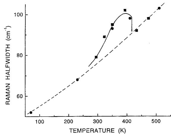
FIG. 5. The temperature dependence of an effective mode width taken at half maximum of the complex band around 260  $\text{cm}^{-1}$ . The dashed line shows an extrapolated monotonic behavior determined by the experimental data beyond the anomalous range where the solid line is merely a guide for the eye.
