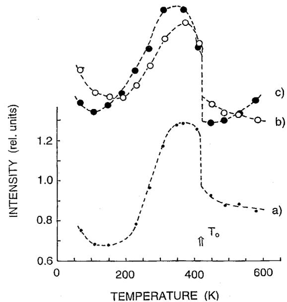
FIG. 4. The temperature dependence of mode intensity in the (ZZ) Raman spectra: (a) integrated intensity (integration in the range from 20 to 400  $\text{cm}^{-1}$ ); (b) an internal vibration at around 260  $\text{cm}^{-1}$  (O–Nb–O bending); (c) an external vibration at about 120  $\text{cm}^{-1}$ . The intensity scale represents an area under the corresponding curves taken after elimination of the population factor by using Eqs. (1) and (2).
